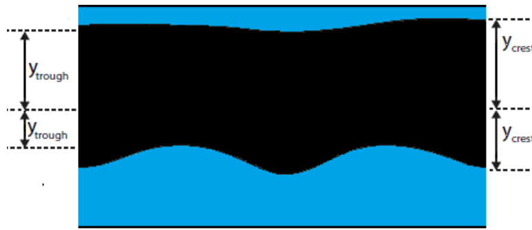
Figure 2.4: Trough and crest of the waves at the bottom and top interface of a slice through the length of the pipe.
