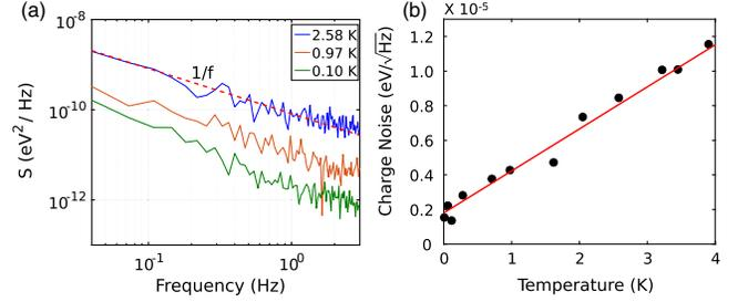
FIG. 4. (a) Charge noise spectra obtained for three different temperatures. At higher frequencies the  $1/f$  signal is masked by white noise. (b) Charge noise at a frequency of 1 Hz as a function of temperature fitted with a linear function.
