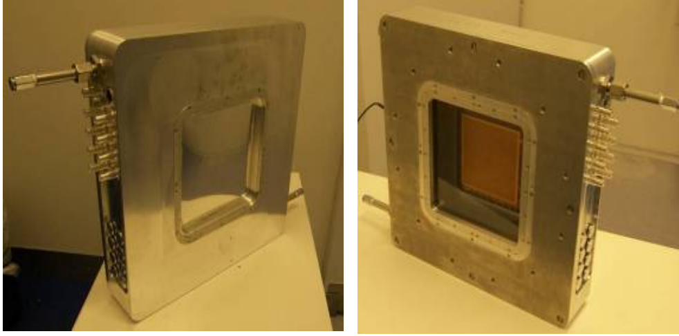
Figure 3.3 On the left, the entrance window side of the scintillating GEM detector. On the right, exit window side of the chamber. Through the glass window, GEM 2 can be seen.
