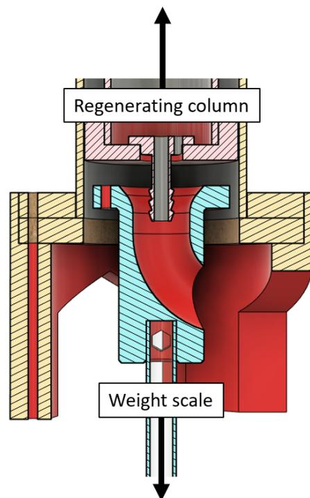
Figure 6.8: Cross-section of the interface part of the regenerating column, enabling it to be seated within the heater, fully resting on the weight scale, while providing connectivity and stress-relief options for connecting hoses and cables.
