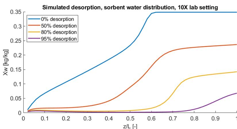
Figure 8.7: Water distribution at various stages of desorption for 10X lab setting. See E.2 for 3X data.
