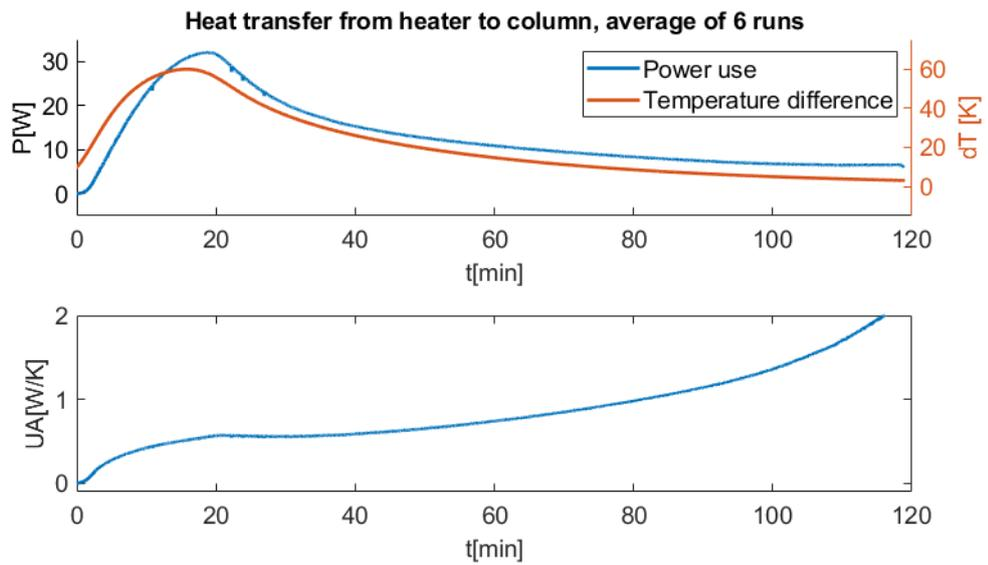
Figure E.5: Approximated heat transfer from the heater to the column.
