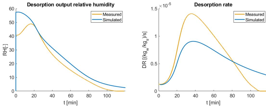
Figure 7.5: Desorption breakthrough curves, relative humidity and gas water content.
