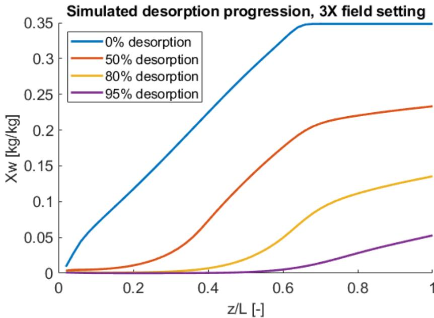
Figure E.3: Water distribution at various stages of desorption
