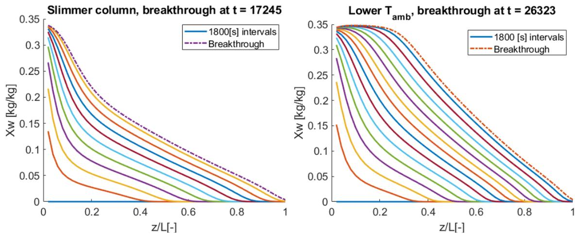
Figure 7.8: Sorbent water distribution during simulated adsorption until breakthrough, with intervals of  $t=1800[s]$ , with an extra line at the moment of breakthrough.
