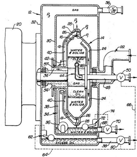
Figure 3.2: Brown and Erickson, also in 1976, utilise a centrifugal approach, with an elaborate internal design to extract the various components from the rotating barrel. Reprint from [15]
