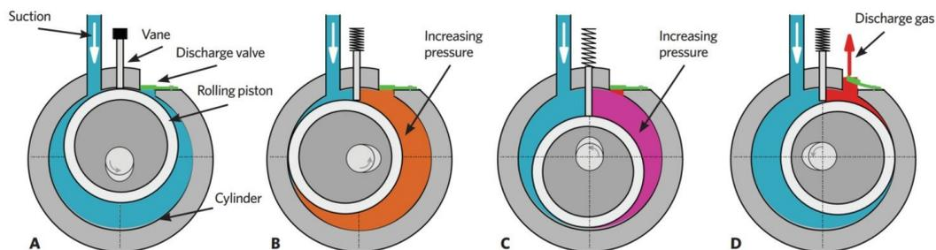
Figure 3.5: Schematic view of a rotary piston compressor at various stages of the compression cycle, reprint from [28].
