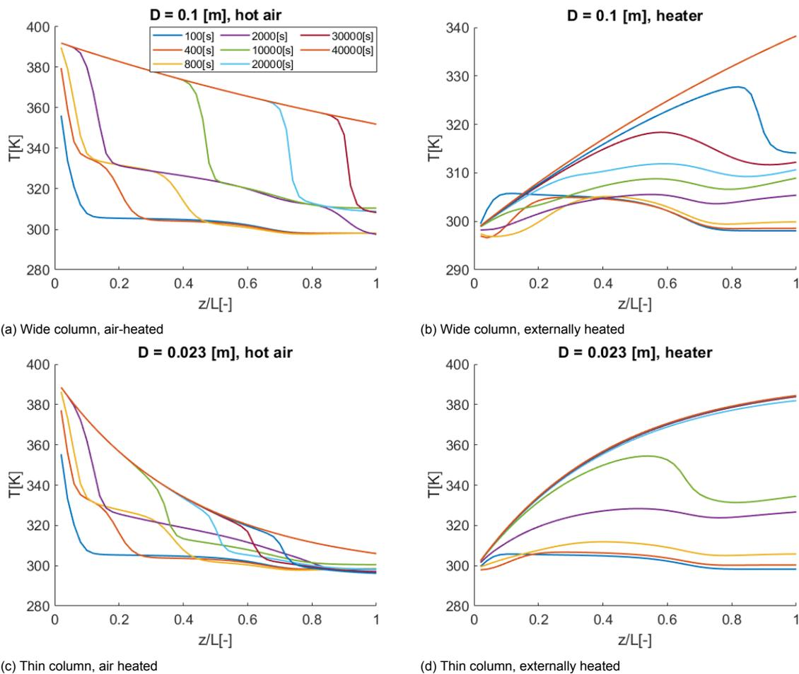
Figure 5.10: Heat distribution curves at selected times during desorption by varying heat sources and diameters. Note how the hot air creates a moving front, similar to the adsorption, while the external heater desorbs along the length of the column.
