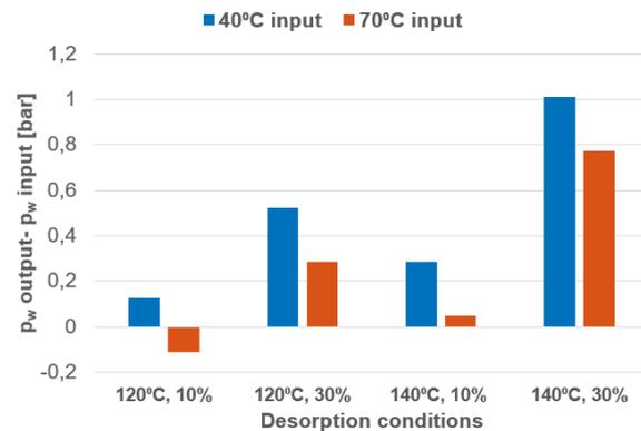
Figure 6.3: Drying potential at a selection of potential input and regeneration conditions (table 6.1)
