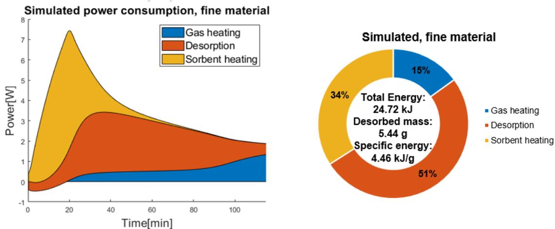
Figure 7.13: Total energy usage of the 3 most relevant categories of simulated data using the fine desiccant.
