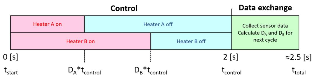
Figure 6.5: Illustration of the control scheme of the ZEF PCB
