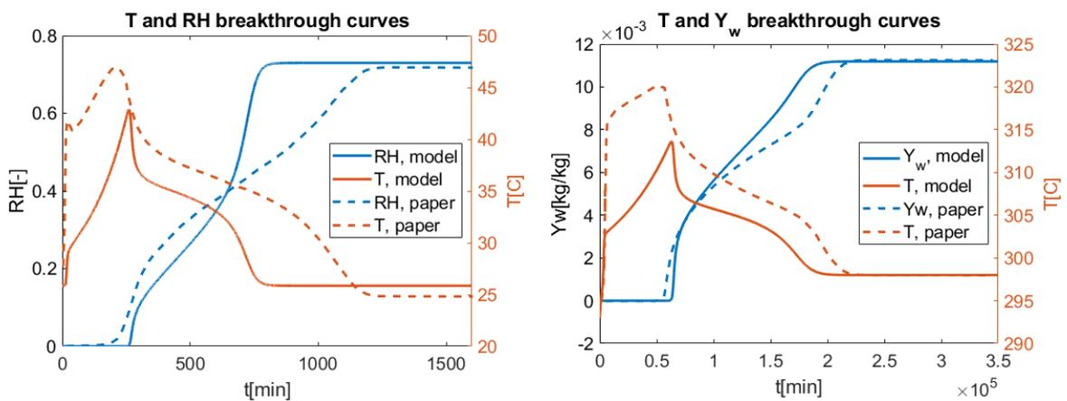
Figure 5.7: Temperature and gas breakthrough curves compared to literature scenarios. Left: this work and Park & Knaebel [62]. Right: this work and Nastaj & Ambrozek [58].
