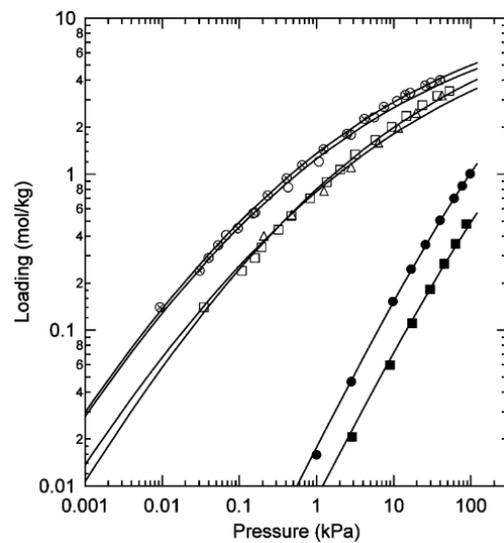
Figure 3.20: Toth isotherms of H<sub>2</sub>O (left) and CO<sub>2</sub> (right) for zeolite 13X(○ at 25 °C, △ at 50 °C), zeolite 5A(◻ at 25 °C, ◻ at 50 °C) and silica gel (● at 25 °C, ■ at 50 °C). Reprinted from [92]
