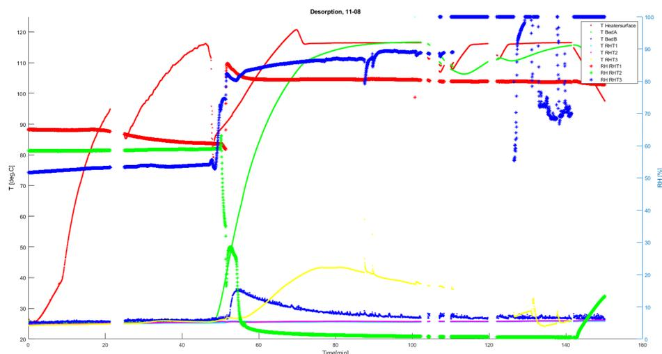
Figure D.4: Rough data of proof of concept experiment. The blank parts indicate a software failure, data has been placed back together via timestamps, note that the erratic behaviour of the RH RHT3 data is indicative of liquid water present on the sensor.
