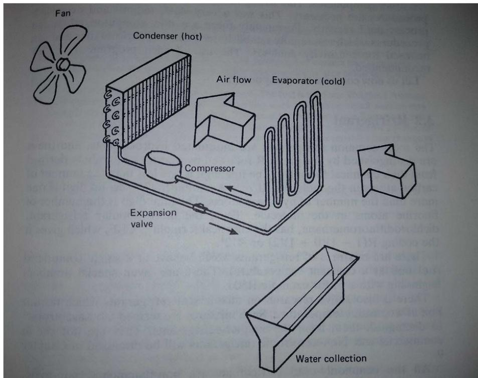
Figure 3.11: Schematic of a refrigeration dehumidifier. Reprinted from [16]
