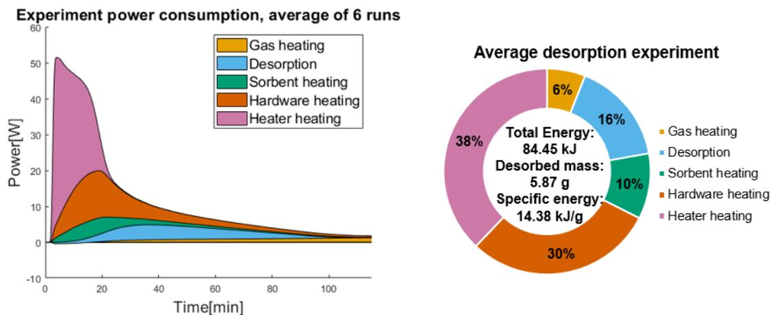
Figure 8.3: Overview of the energy consumption of the desorption experiment.
