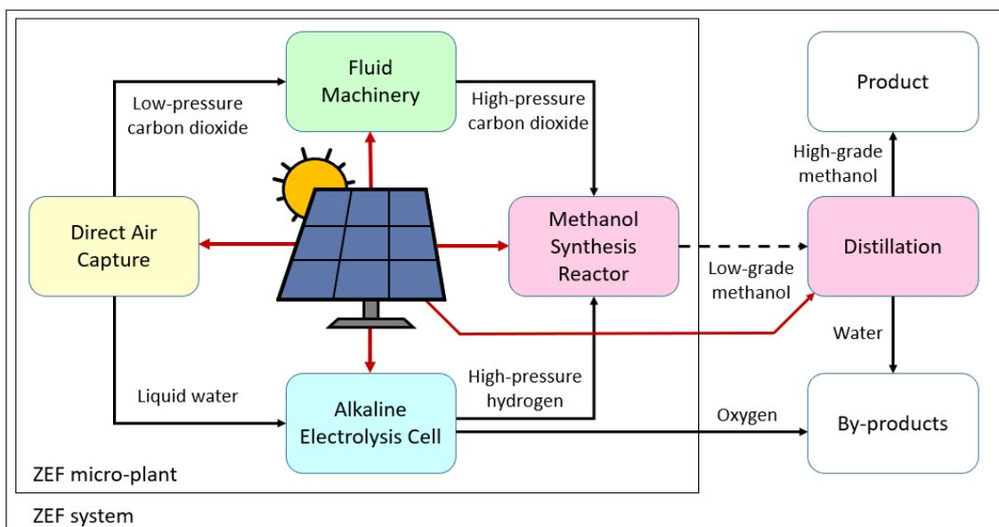
Figure 1.6: Simplified overview of the ZEF concept, powered by solar PV.
