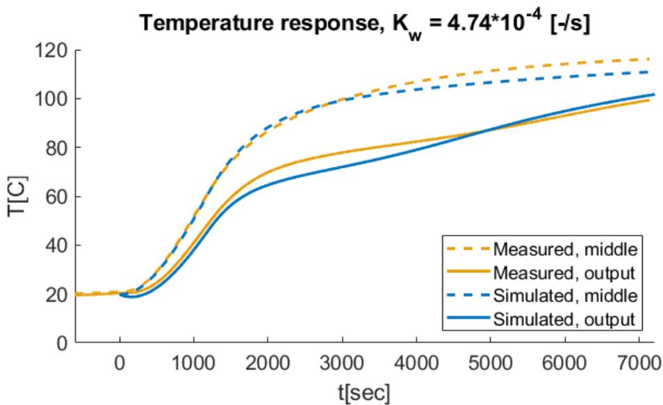
Figure 7.4: Temperature response of the experiment with the fitted mass transfer coefficient
