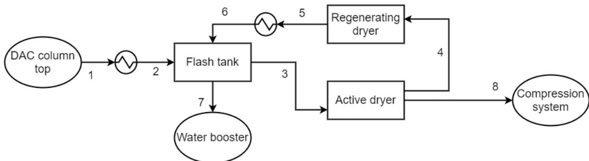
Figure 8.2: Simplified schematic of the closed loop concept.
