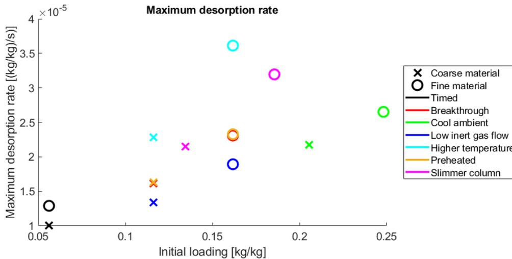
Figure 7.14: Maximum desorption observed and average breakthrough column loading in the simulated data from the described scenarios.
