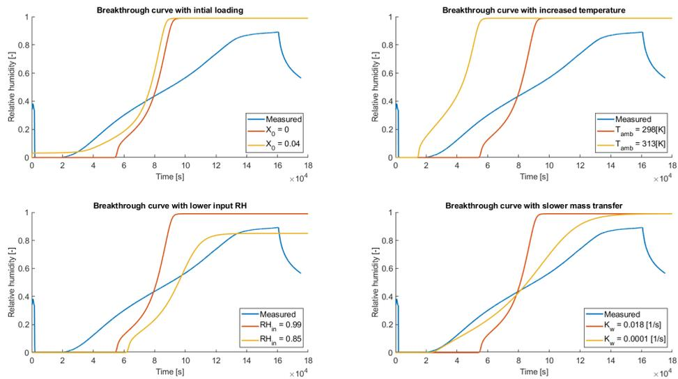
Figure 6.17: Variations of breakthrough data modelled in figure 6.16 and compared to measured data.
