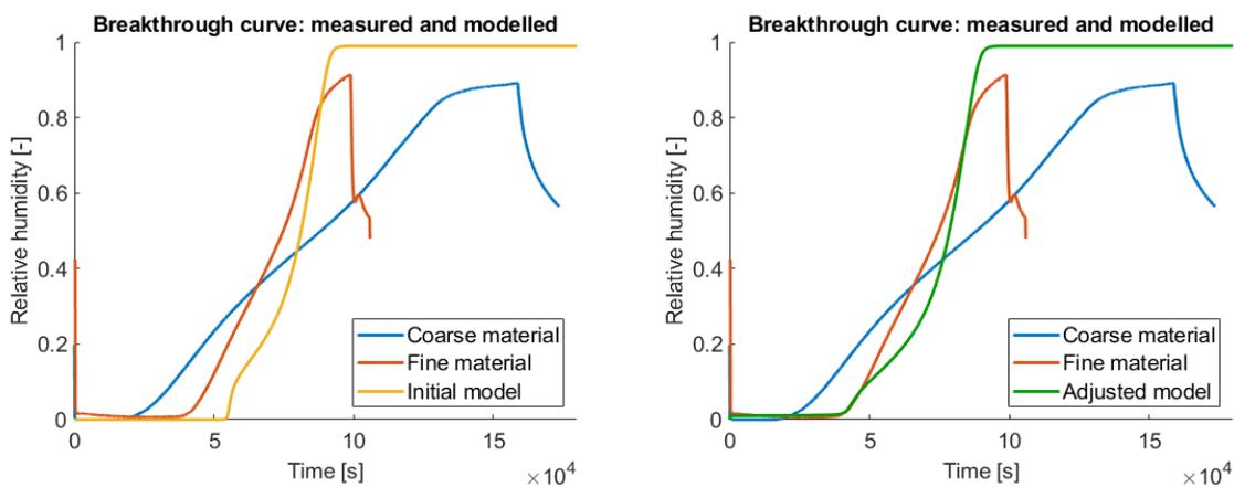
Figure 6.18: left: Breakthrough data of fine material, compared to coarse material and model. Left: model such as presented in figure 6.16 Right: model with  $X_0 = 0.025$ [kg/kg] and  $K_w = 0.0036$  [1/s]
