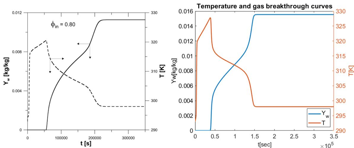
Figure 5.3: Temperature and breakthrough curves, with all known parameters identical. Left: Nastaj & Ambrozek, 2009 [58]. Right: This work.
