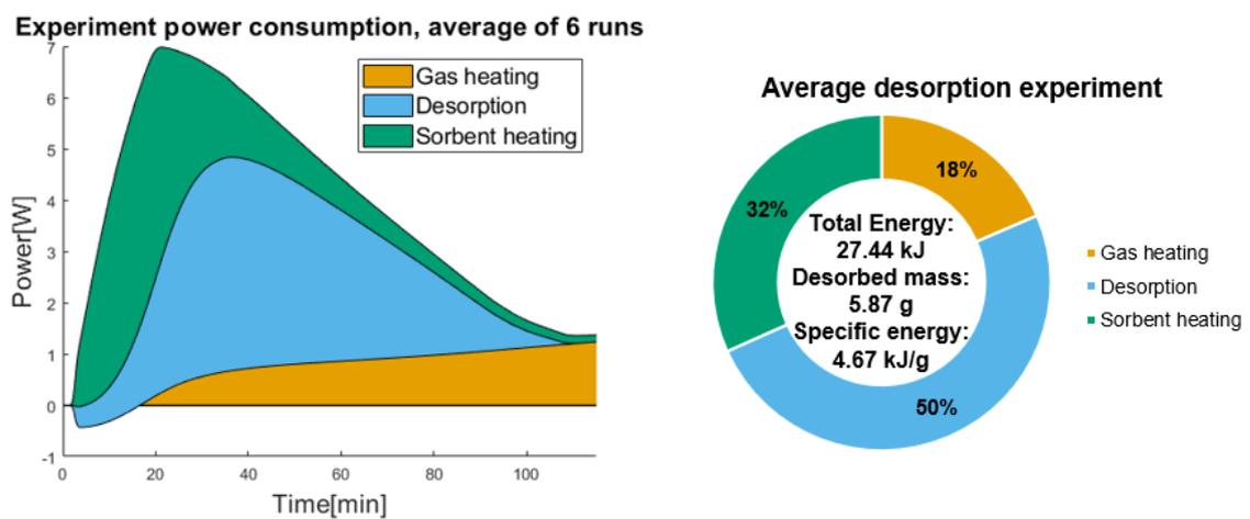
Figure 7.11: Total energy usage of the 3 most relevant categories of the averaged data from all desorption experiment runs.
