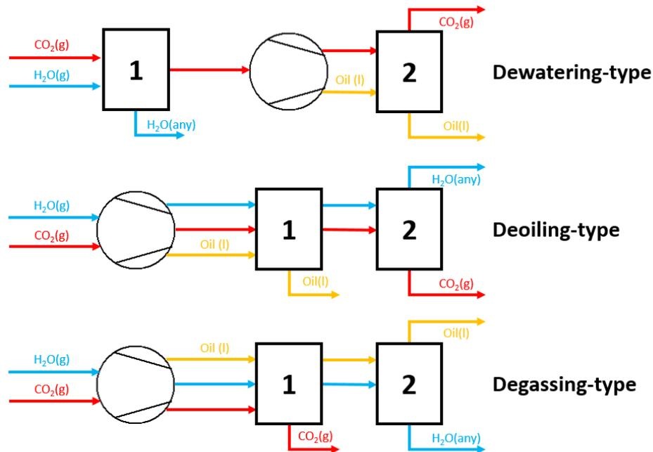
Figure 8.1: The three device types as identified in chapter 3
