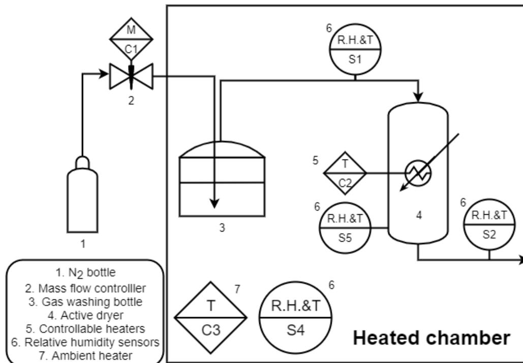
Figure 6.12: PFD for the breakthrough experiment
