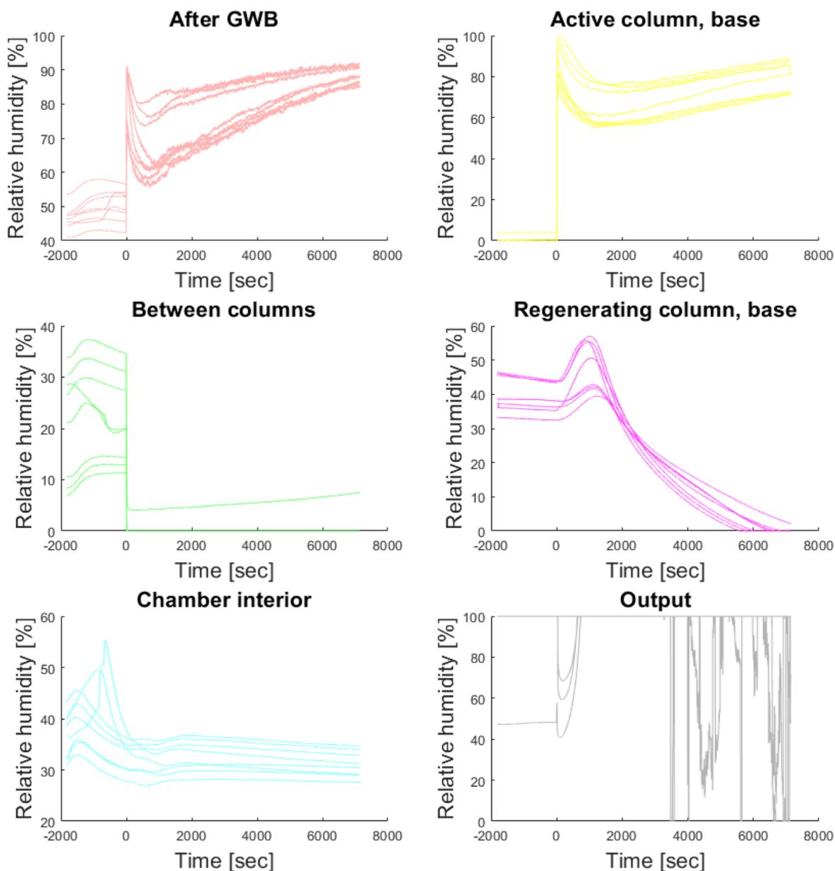
Figure D.5: Relative humidity at various positions during all desorption experiment runs
