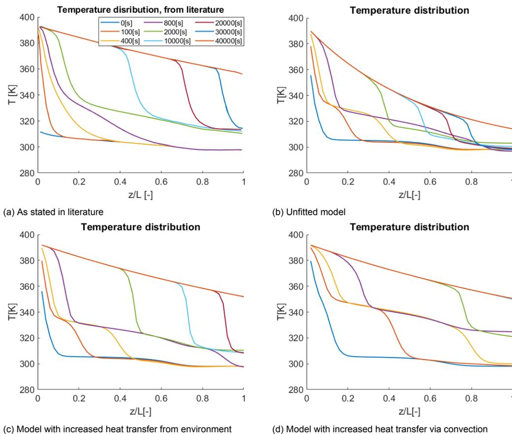
Figure 5.8: Heat distribution curves at specific times comparing literature (a) with an unfitted model (b) and 2 variations (c and d)
