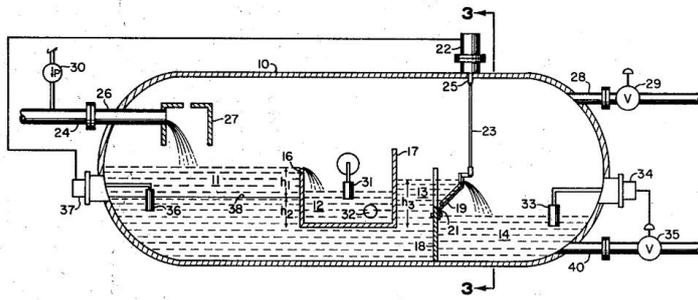
Figure 3.1: Peters' three-phase separator from 1976 takes a settling-based approach, using many components to control fluid levels in the various compartments of the system. Reprint from [67]
