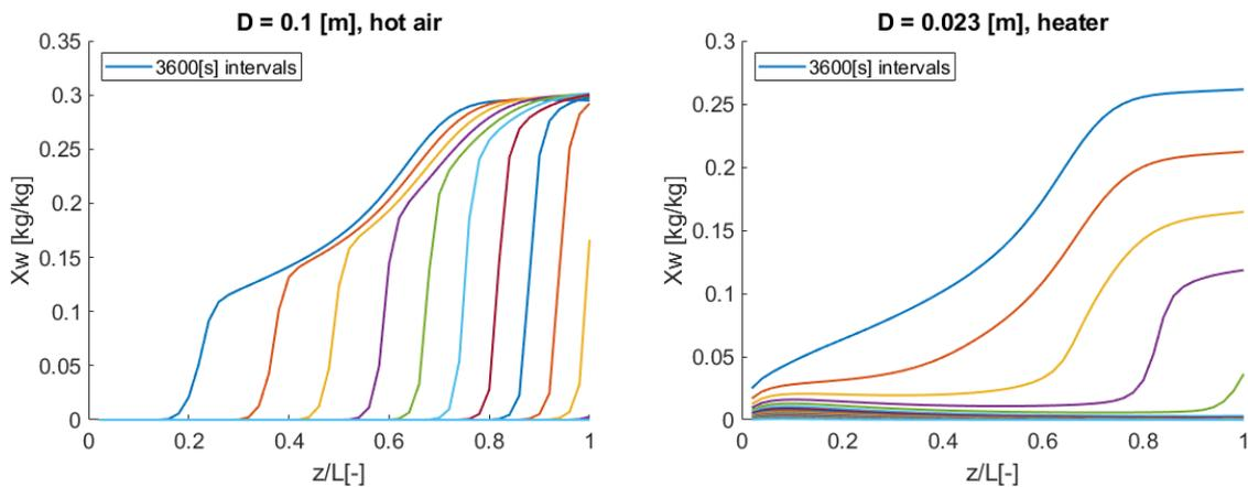
Figure 5.11: Sorbent water content distributions at intervals of  $t = 3600[s]$ , figures are made from the same model runs as E.1a and E.1d respectively.
