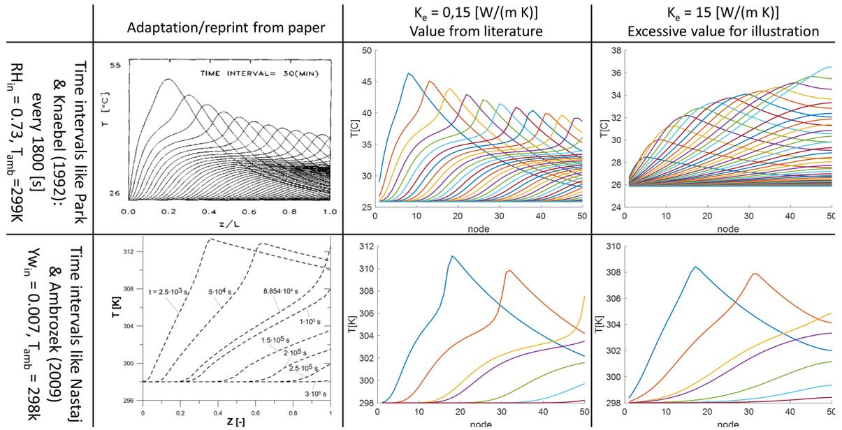
Figure 5.4: Emulation of temperature-space curves at specific intervals from Nastaj & Ambrozek (2009) and Park & Knaebel (1992), as well as a purposeful exaggeration to illustrate the difference between the model, and to highlight the thermal conductivity discrepancy.
