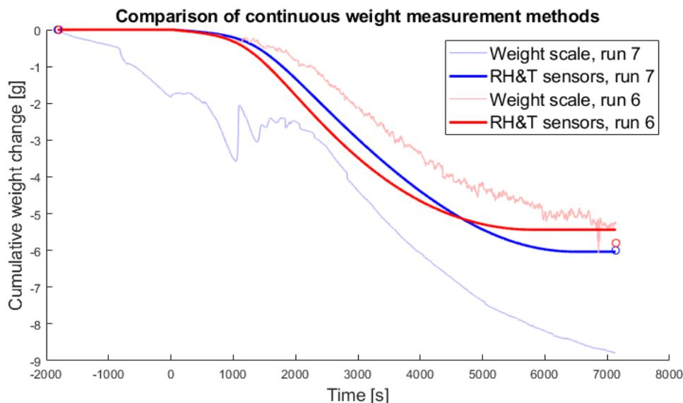
Figure 6.15: Illustrative examples of the two weight measurement methods.
