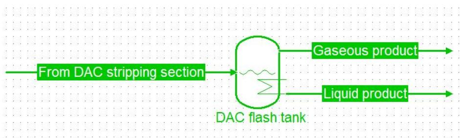
Figure 2.2: The COCO simulator model of the DAC flash tank
