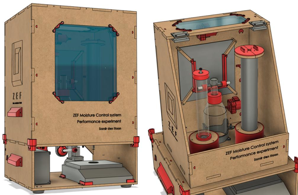
Figure 6.9: Left: CAD model of the machine's assembly. Right: The equipment inside the chamber is displayed by hiding the hood and top-hinging door of the CAD model.
