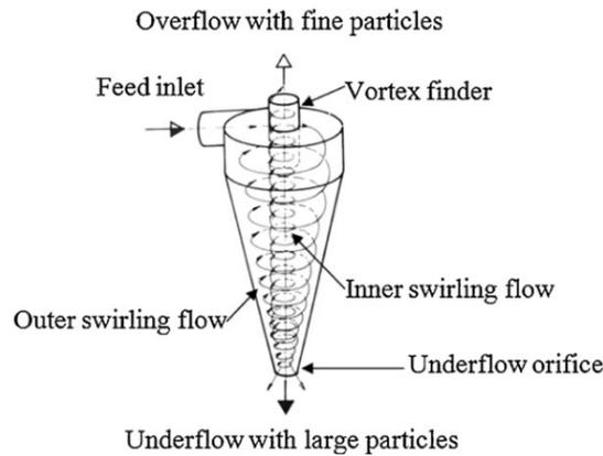
Figure 3.12: Schematic of a typical hydrocyclone. Reprint from [83].
