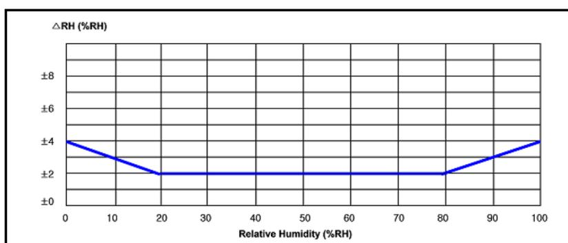
Figure 8.6: Telaide's ChipCap2 datasheet report a lower RH accuracy at very high and very low RH, which is common for these type of sensors [85].
