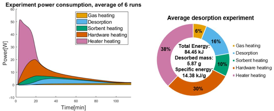
Figure 7.10: Total energy usage of the 5 most relevant categories of the averaged data from all desorption experiment runs.
