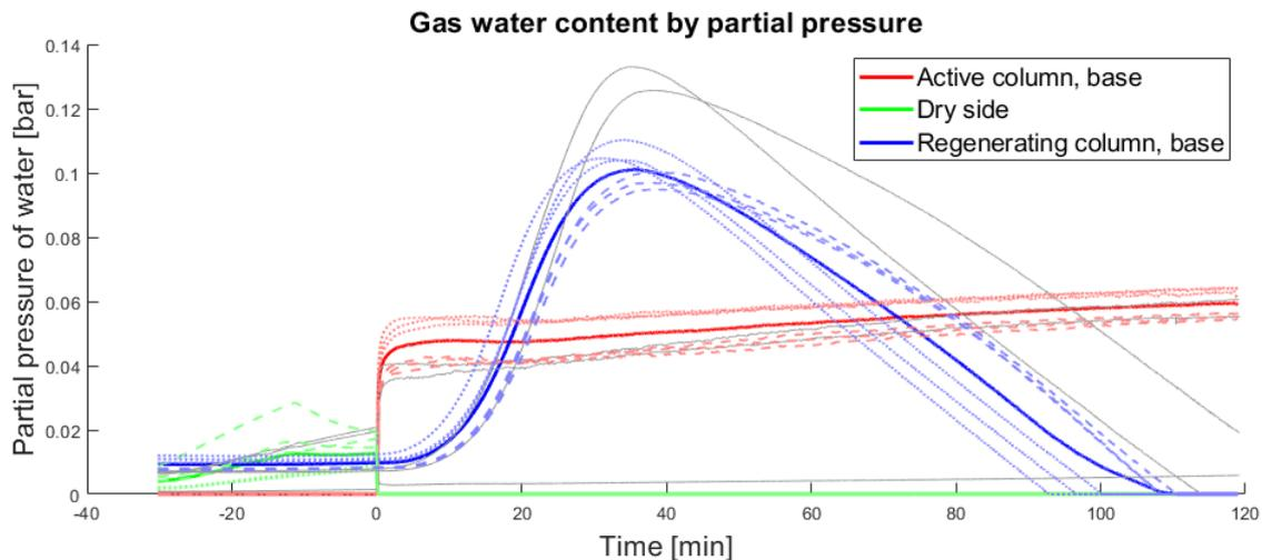
Figure 6.14: Gas water content at various points in the experiment. Note that the gas flow is switched on at  $t=0$ .
