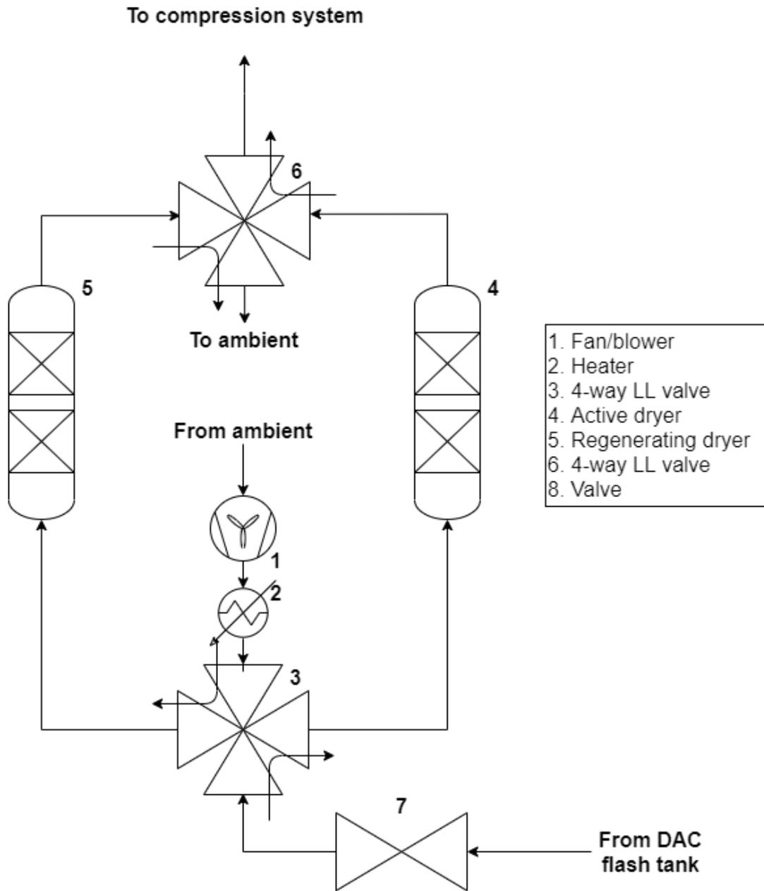
Figure A.1: PFD of the double-column concept setup
