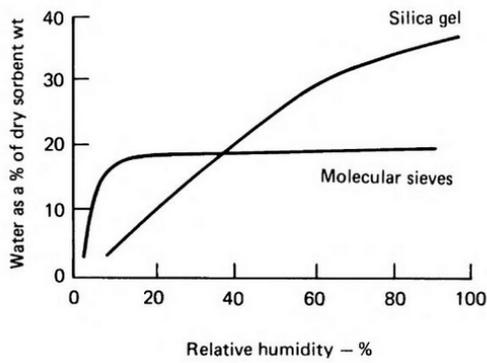
Figure 3.18: "Illustrative equilibrium characteristics for two common sorbents", reprint from [16]
