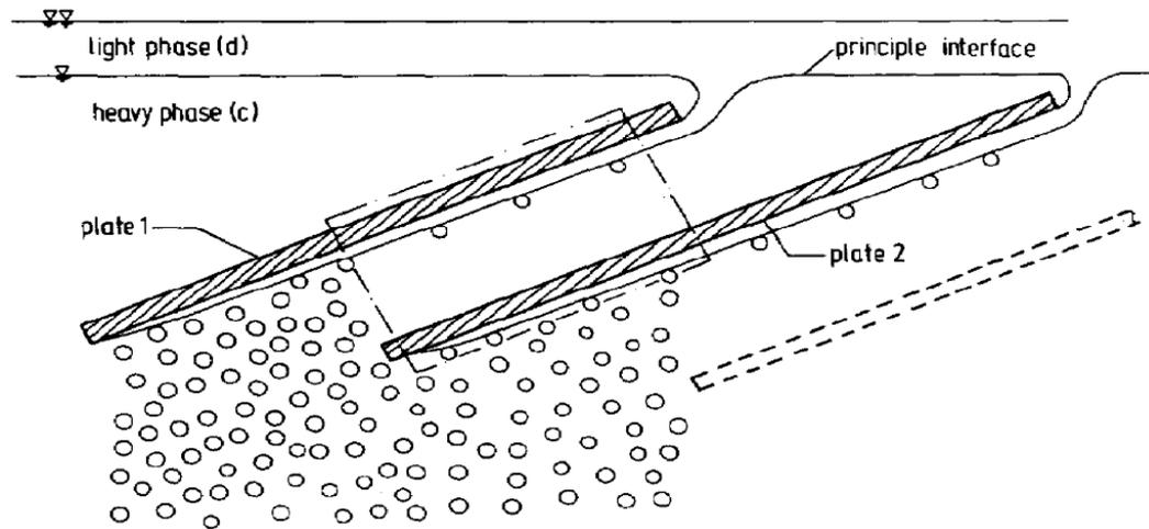
Figure 3.10: Illustration of the principle of plate coalescence. Reprint from [74]
