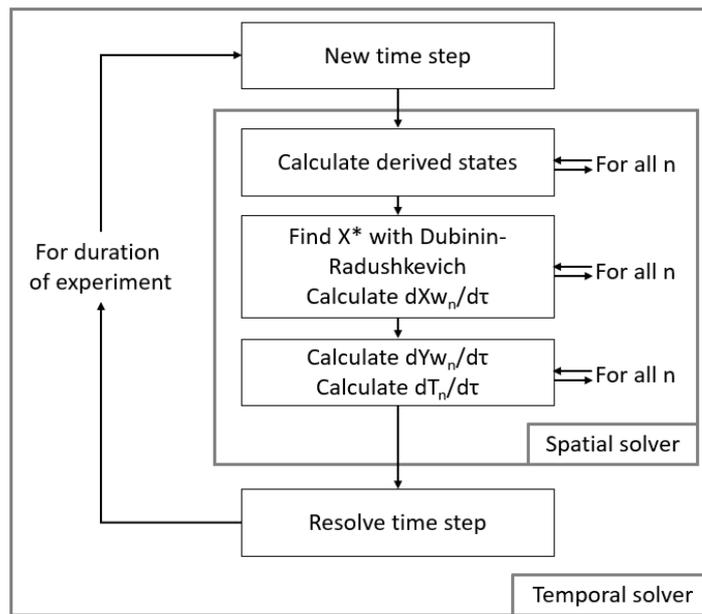
Figure 5.1: Sketch of an algorithm that depicts the interrelation of the model equations.
