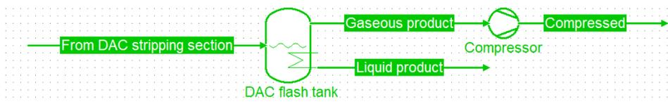
Figure 3.8: The COCO simulator model used to find the dewpoints of various compressed  $CO_2$  and  $H_2O$  mixtures.
