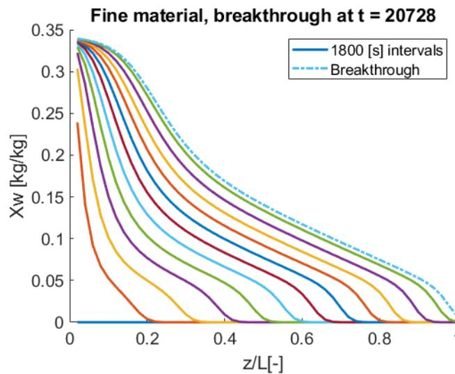
Figure 7.9: Sorbent water distribution during alternative simulated adsorption until breakthrough, with intervals of  $t=1800[s]$ , and an extra line at the moment of breakthrough
