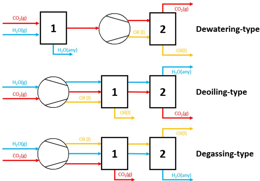
Figure 3.4: The three possible configuration types of the moisture control system: dewatering (DW), deoiling(DO) and degassing(DG).
