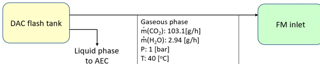
Figure 2.3: Overview of the inlet conditions of the FM section
