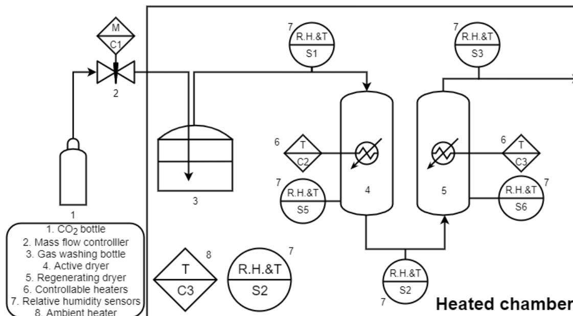
Figure 6.11: PFD for the desorption experiment
