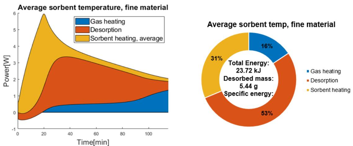
Figure E.2: Energy usage of simulated data when average temperature is used, instead of temperature measured at one node.
