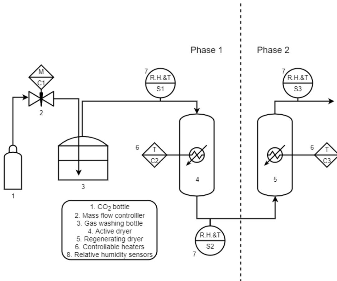
Figure 6.4: PFD of the experimental concept
