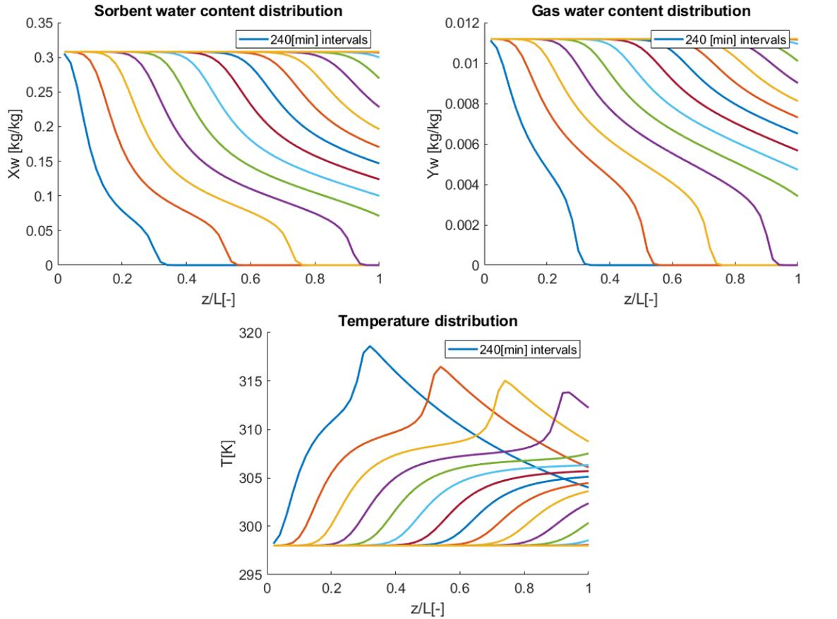
Figure 5.6: The three main states at intervals of 240[min]. Conditions identical to the right side of figure 5.7
