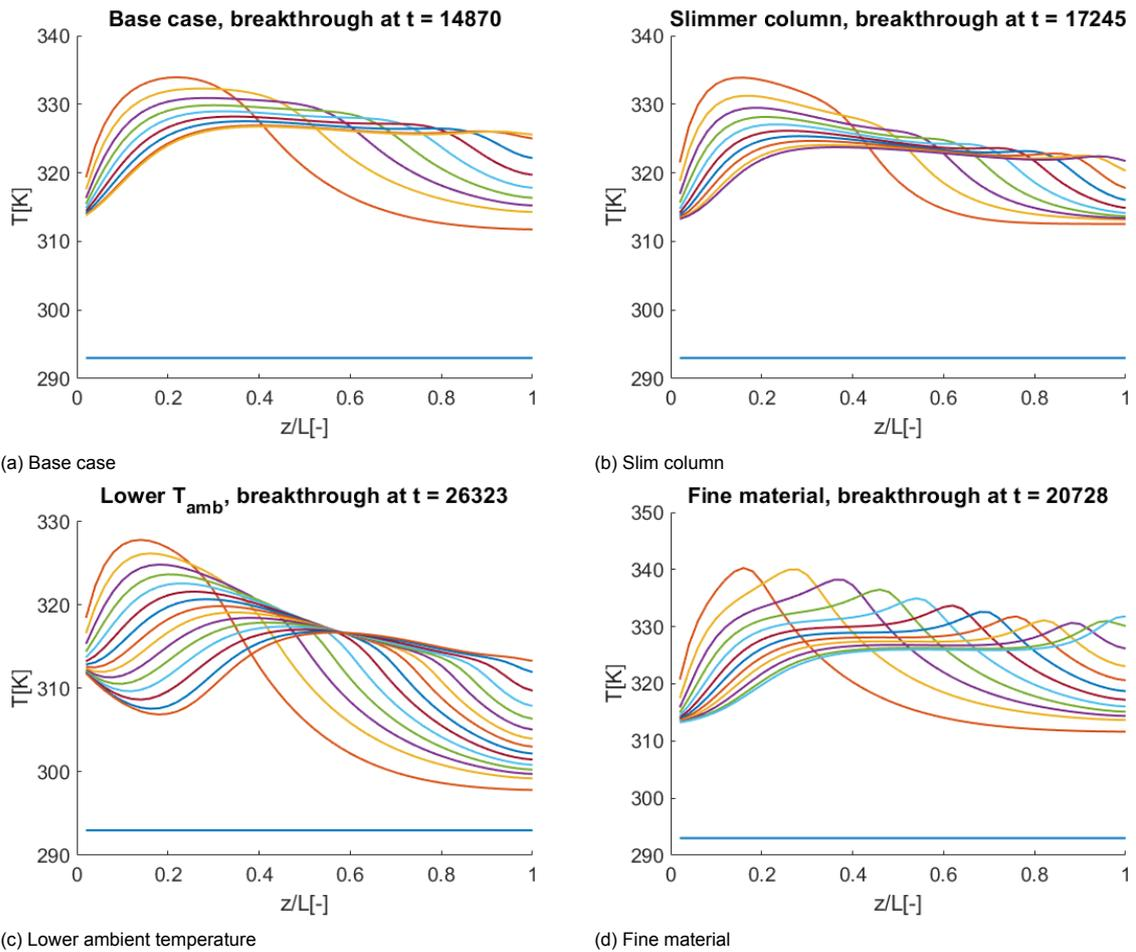
Figure E.1: Adsorption until breakthrough, space temperature curves of the scenarios sketched in figures 7.7, 7.8, 7.9. Lines with intervals of  $t=1800[s]$
