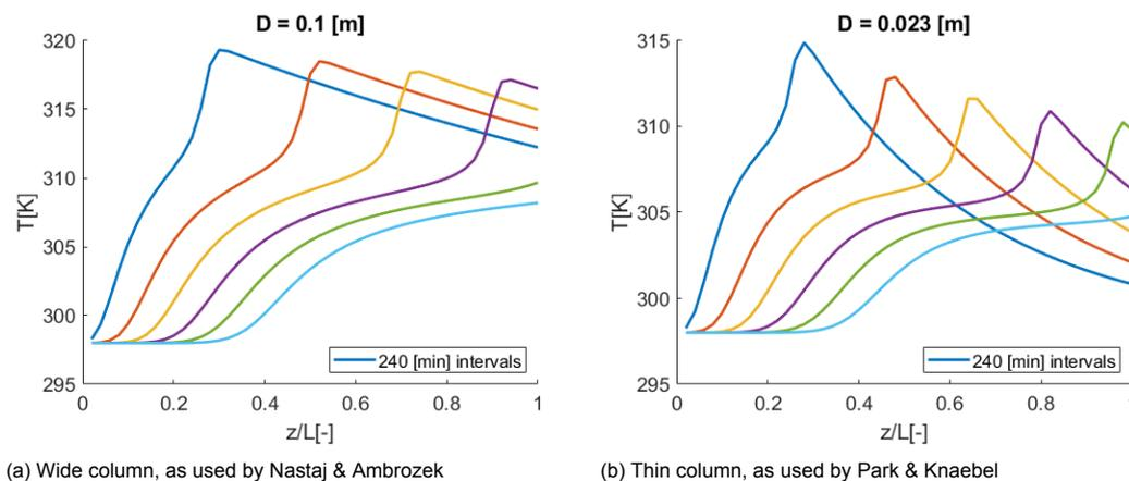
Figure 5.9: Temperature distributions at intervals of  $t = 240$  [min] to illustrate effect of column diameter. Modelling conditions like 5.8c.
