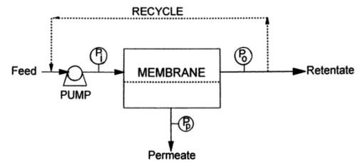
Figure 3.15: Overview of a cross-flow filtration system. Reprint from [20].
