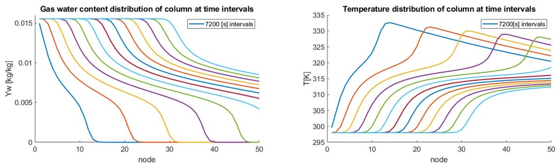
Figure 5.2: Gas water content and temperature distributions within the column at identical time intervals of 7200 [s]
