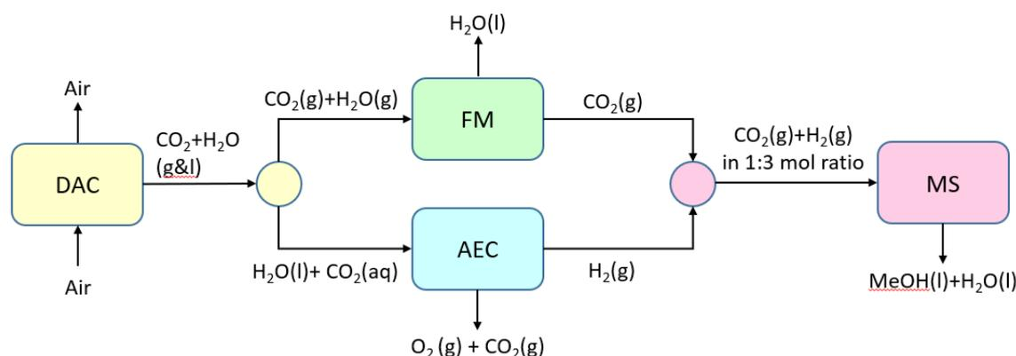
Figure 2.1: Simplified schematic of the ZEF micro-plant
