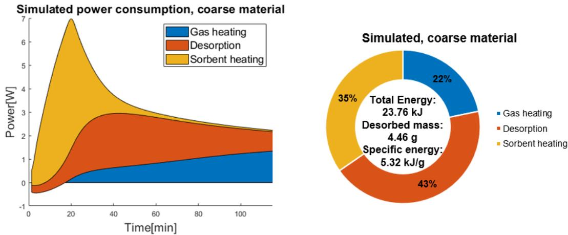
Figure 7.12: Total energy usage of the 3 most relevant categories of simulated data using the coarse desiccant.
