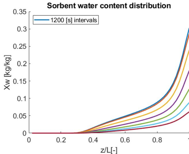
Figure 7.6: Sorbent water distribution during simulated desorption experiment, with intervals of 1200[s]
