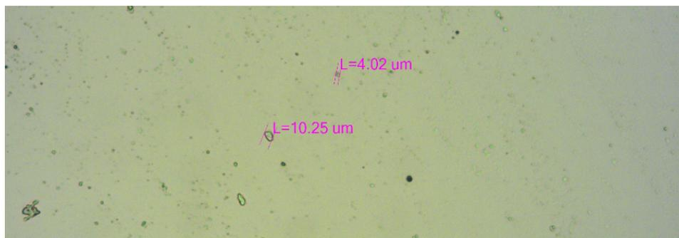
Figure 3.9: Emulsion formed from compressor exhaust during early testing at ZEF, as seen under a basic lab microscope.
