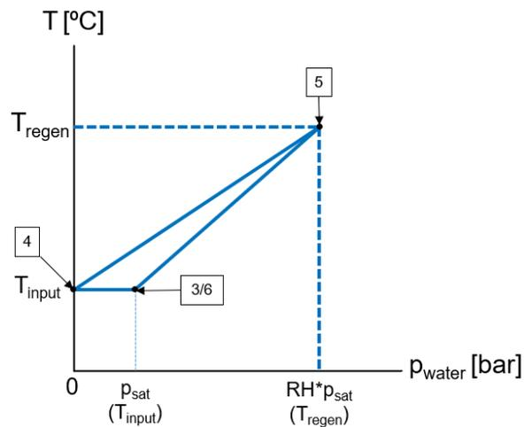
Figure 6.2: Illustration of possible water content in MCS cycle. Values for potential in- and output conditions in table 6.1. Flow labels according to figure 6.1
