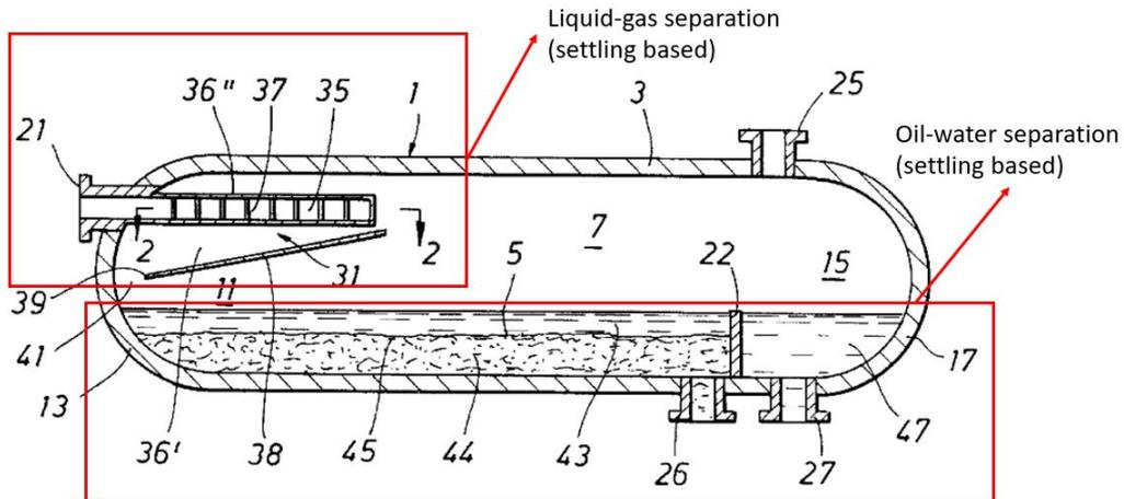
Figure 3.3: Polderman's 2003 design is simpler than the earlier examples, making it easier to see that this three-phase separator consists of two separators in series. Adapted from [70]
