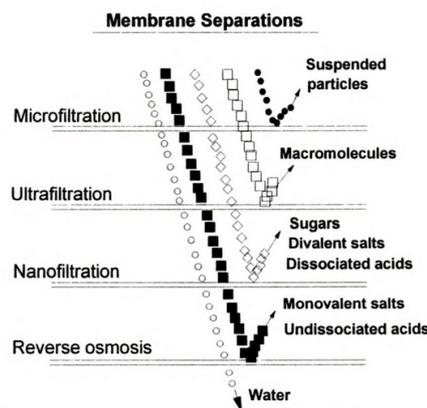
Figure 3.13: Various types of filtration processes. Reprint from [20]
