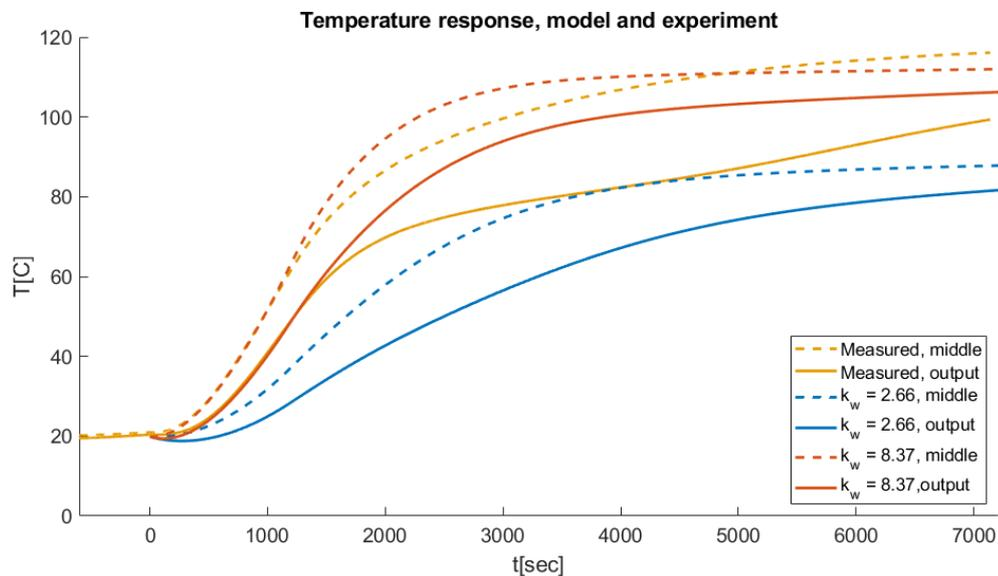
Figure 7.2: Temperature response of the experiment and model with two heat transfer coefficients.
