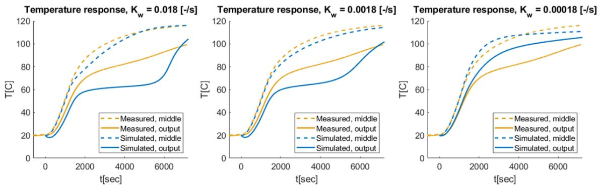
Figure 7.3: Temperature response of the experiment and model with varying mass transfer coefficients.
