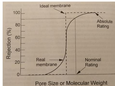
Figure 3.16: Illustration of non-idealities and nominal ratings of ultrafiltration membranes. Reprint from [20]
