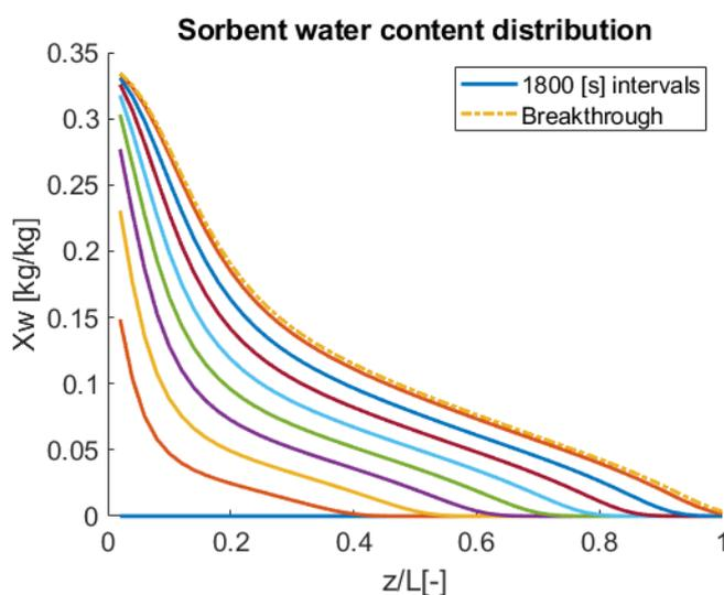
Figure 7.7: Sorbent water distribution during alternative simulated adsorption until breakthrough, with intervals of 1800[s], and an extra line at the point of breakthrough at  $t = 14870$ [s]
