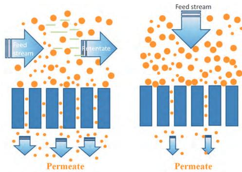
Figure 3.14: Schematic of cross-flow and dead-end filtration configurations. Reprint from [29]
