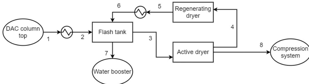
Figure 6.1: Illustration of the working principle of the looped-column setup. A PFD of this concept can be found in appendix A.1
