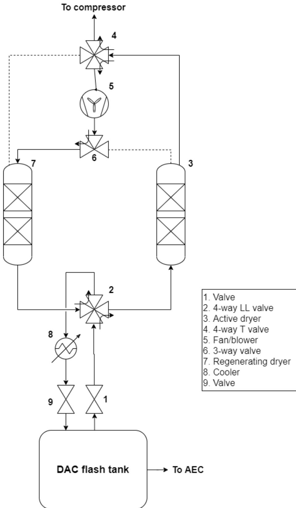
Figure A.2: PFD of the looped-column concept setup
