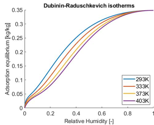
Figure 3.19: Several isotherms for silica gel using the Dubinin-Radushkevich equation and parameters from [58]
