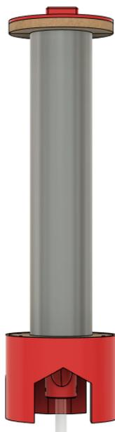
Figure 6.7: Assembly that is used to house the regenerating column. The column can be placed by removing the lid. The assembly is fitted with a silicone heater ribbon and rockwool isolation sleeve that is not depicted on this image.
