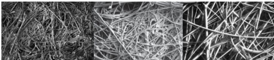
Figure 3.17: Materials for Parker Hannifin Corporation coalescing filters, 500x magnification. Left: grade 2, middle: grade 4, right: grade 8. Adapted from [63]
