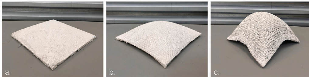
Fig. 2. Knitted textiles with distinct knit architectures deforming differently under the same concrete load: (a) Cross miss pattern; (b) Single cross tuck pattern; (c) Double half cardigan pattern. Project and photos by Lucy Flieger [8].
