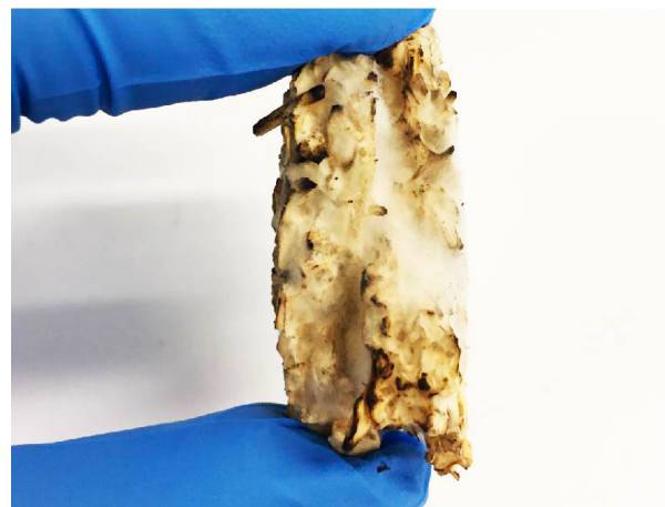
Figure 8. shows Non-living composites can also be healed in the instance where a living inoculum is introduced to the treated composite under the right conditions. Whether we use pure mycelium, in the form of spawn or liquid culture, or inoculated substrates, the process of healing involves certain critical steps such as adding and maintaining moisture and a sterile habitat.
