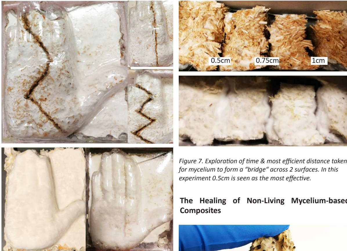
Figure 6. From top left clock wise: 3 different cuts. Then the healed composite after 5 days inside the mould. Lastly the fully healed sample.
