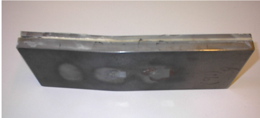
Figure 7-16: Deformation after 3-point bending test
