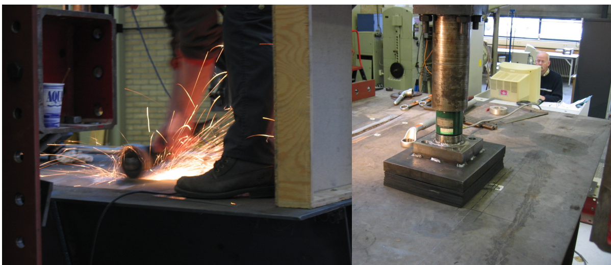
Figure 4-25: Making cracks (left), load application (right)
