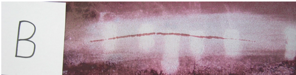
Figure 4-37: Fatigue crack B in test panel A after dye penetrant inspection
