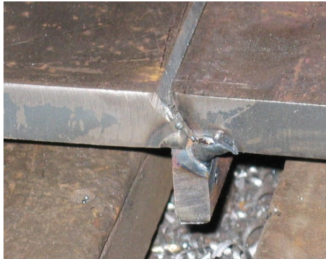
Figure 5-7: Backing strip to simulate trough web
