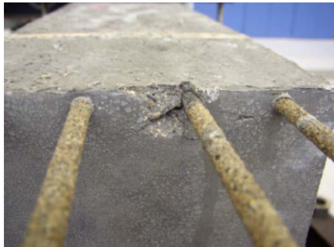
Figure 7-61: Slip failure of CFRP bar in C200, 3 mm concrete cover
