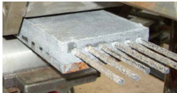
Figure 7-63: CFRP reinforced beam
