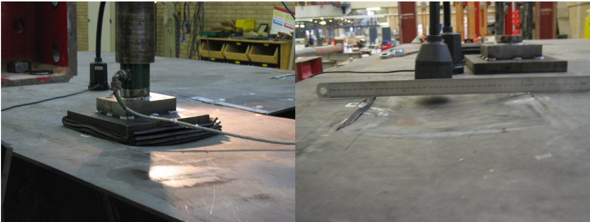
Figure 4-27: Compression at maximum load (left), deformation after unloading (right)
