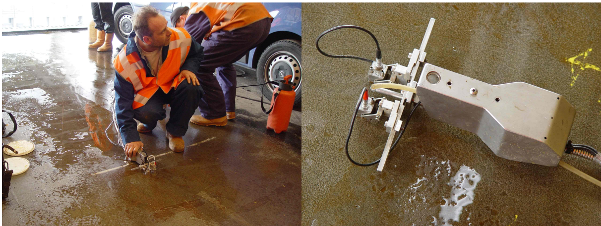
Figure 8-9: TOFD inspection (left), TOFD scanner (right)
