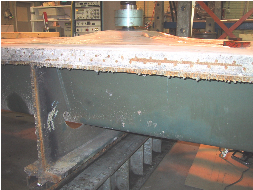
Figure 6-44: Full-scale fatigue test at test panel with RHPC surfacing.
