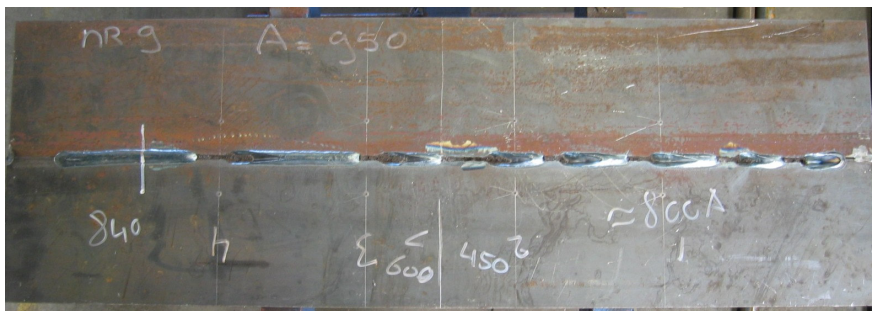
Figure H-4: Topside specimen 9 after welding
