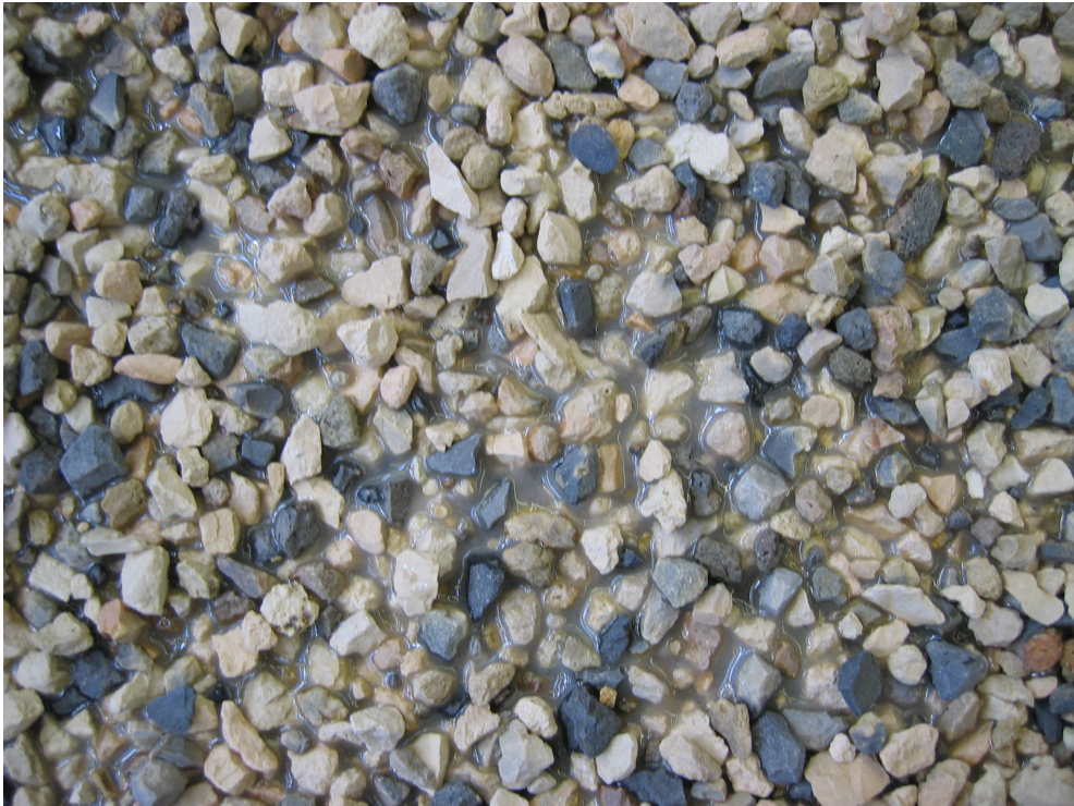
Figure 6-28: Epoxy layer sprinkled with bauxite aggregate on test panel A
