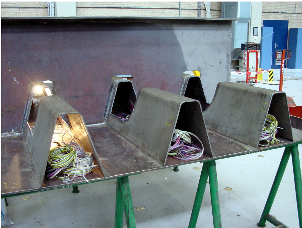
Figure 6-31: Accessibility underside deck plate to attach strain gauges
