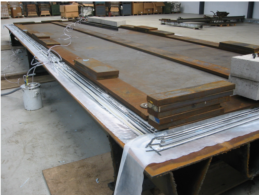
Figure 7-13: Vacuum infusion test on bridge deck section
