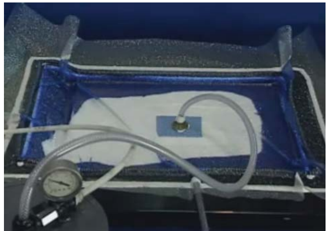
The resin is introduced in the mold and the vacuum assists the impregnation of the reinforcement material. (source: http://www.youtube.com/watch?v=xVErb2-bnuw )
