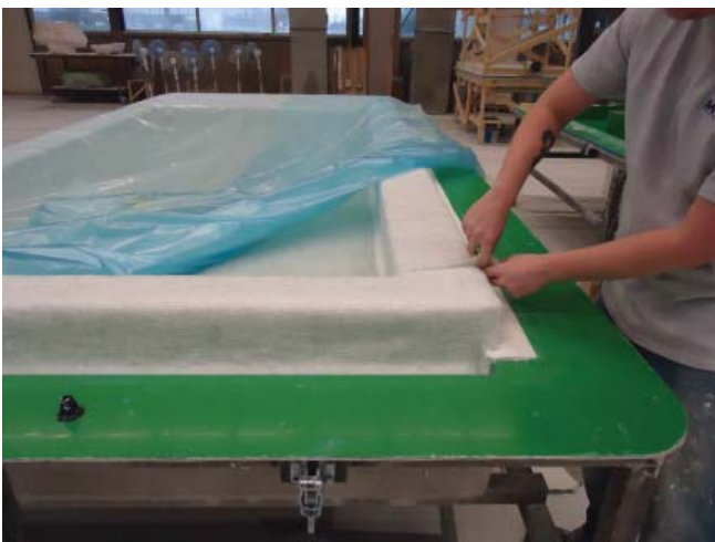
Closed mold production technique of a GRP sandwich element in Polux BV. (source: photo by the author)
