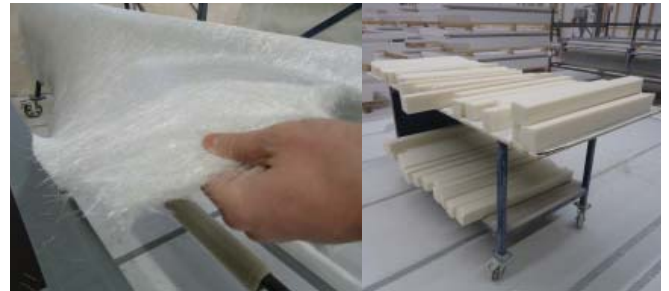
The material used for the distribution of the resin // Foam core material (source: photo by the author)
