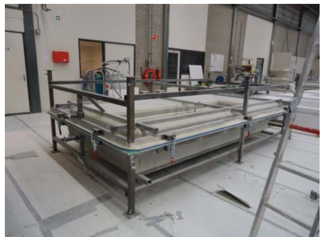
Closed mold during the fabrication of a GRP sandwich element in Polux BV. The resin is let for one day in the mold to cure. After that the element is ready. (source: photo by the author)
