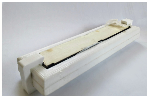
Fig. 4. Clamp used for composite tensile samples.
