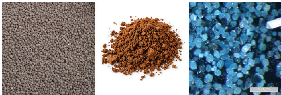
Figure 1-2 Three phosphate recovery minerals in focus: struvite (left [53]), calcium phosphate granules (middle [85]), and vivianite (right [65]).
