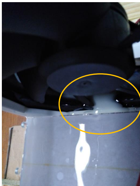
Figure 38: Layer of TEPA displaced by the fan
