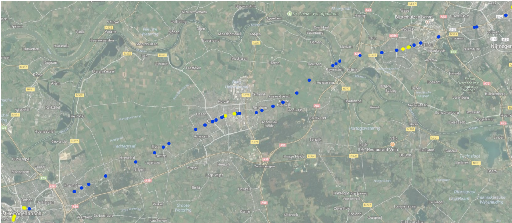
Figure 3.2: Geographic overview of control points (yellow = XYZ for switches, blue = Z for crossings and bridges)
