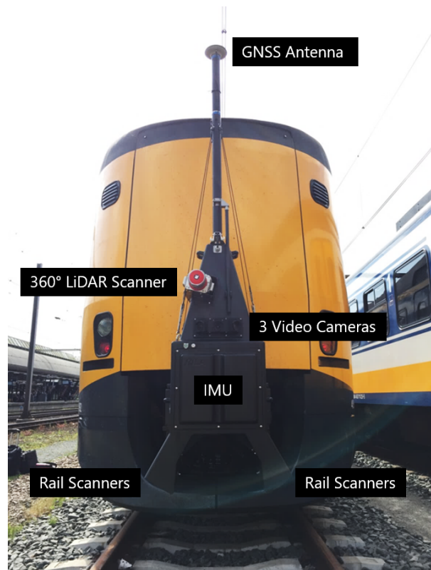
Figure 2.1: Fugro RILA 6.0 system and its components (Credits: Fugro)
