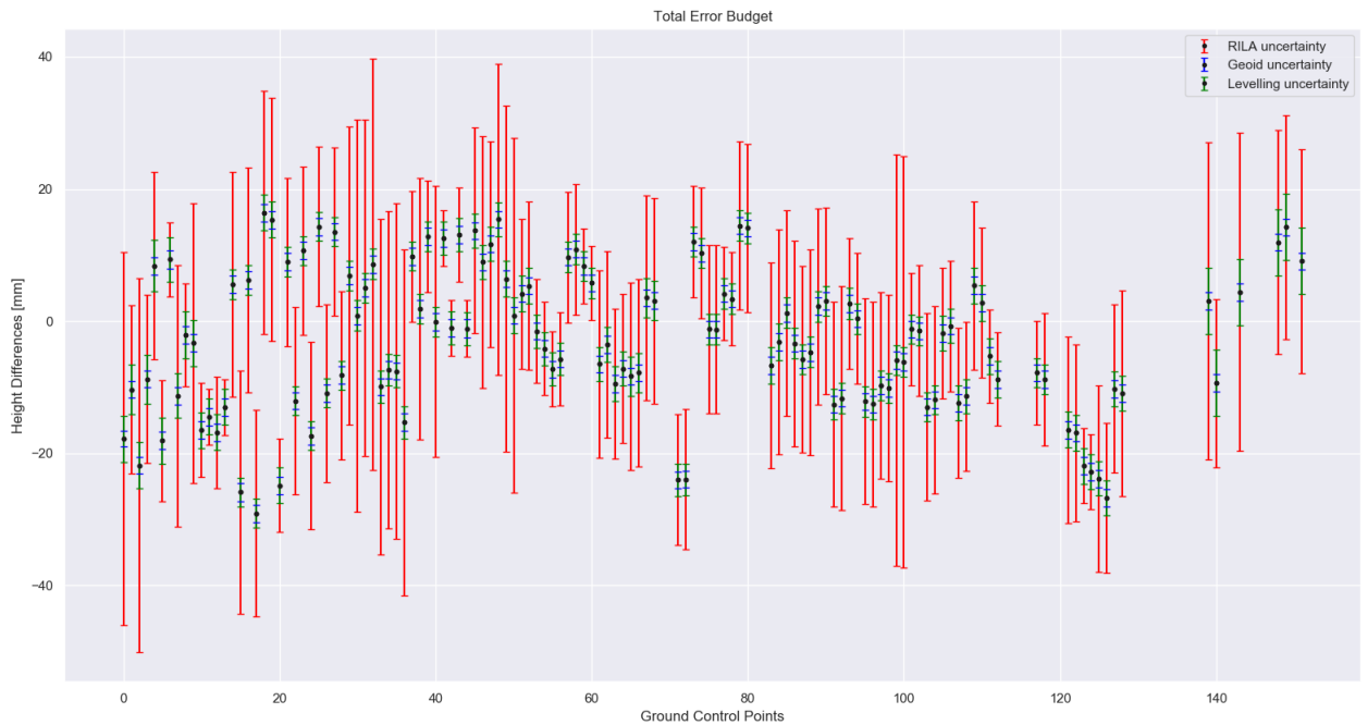
Figure 4.20: Total error budget plotted for each GCP and the height difference. Uncertainties from RILA seem to show the most influence.
