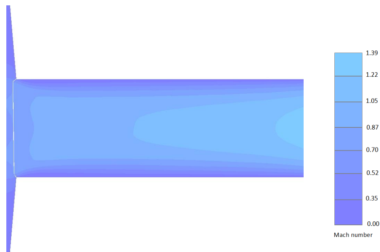
Figure 6.4: Mach number profile in the slit
