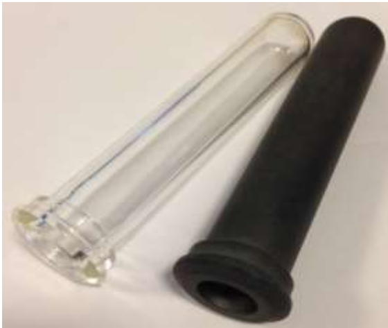
Figure S1. Glass and SiC vials available for the Anton Paar Monowave 300 microwave reactor. Both vials have the same geometry.
