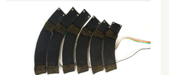
FIG I. 4 Final prototype of the Affective Sleeve made from felt fabric, nitinol wire and elastic bands. Top view when cuffs are unfastened.
