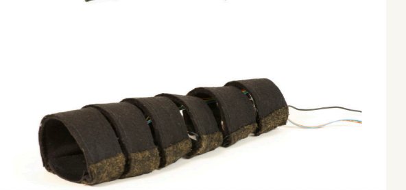
FIG I. 5 Final prototype of the Affective Sleeve made from felt fabric, nitinol wire and elastic bands. Perspective view when cuffs are fastened.
