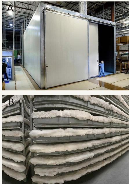
Figure 4: Production of pure mycelium foams (Vandelook et al., 2021)
