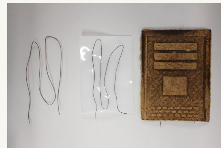
Figure 37: Separate SMA wire, wire in silicon and wire in fungal textile
