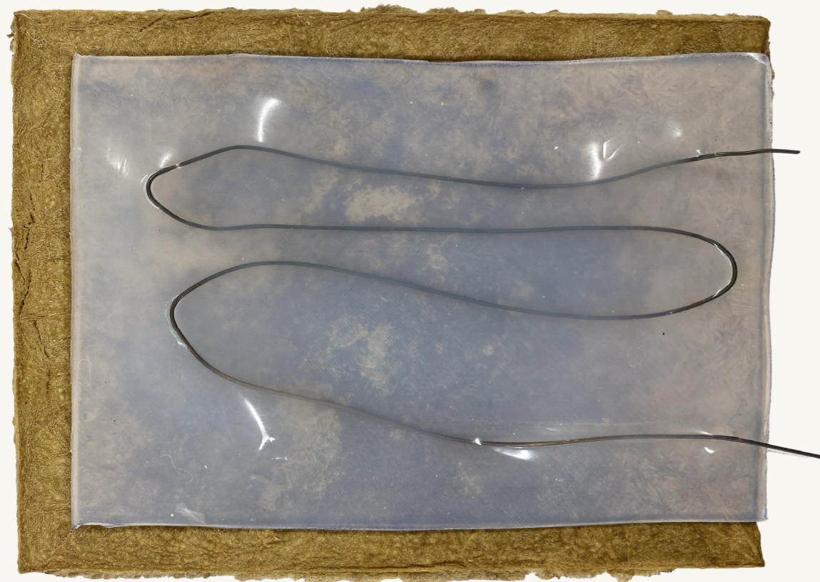
Fungal textile layer + silicon with SMA layer
