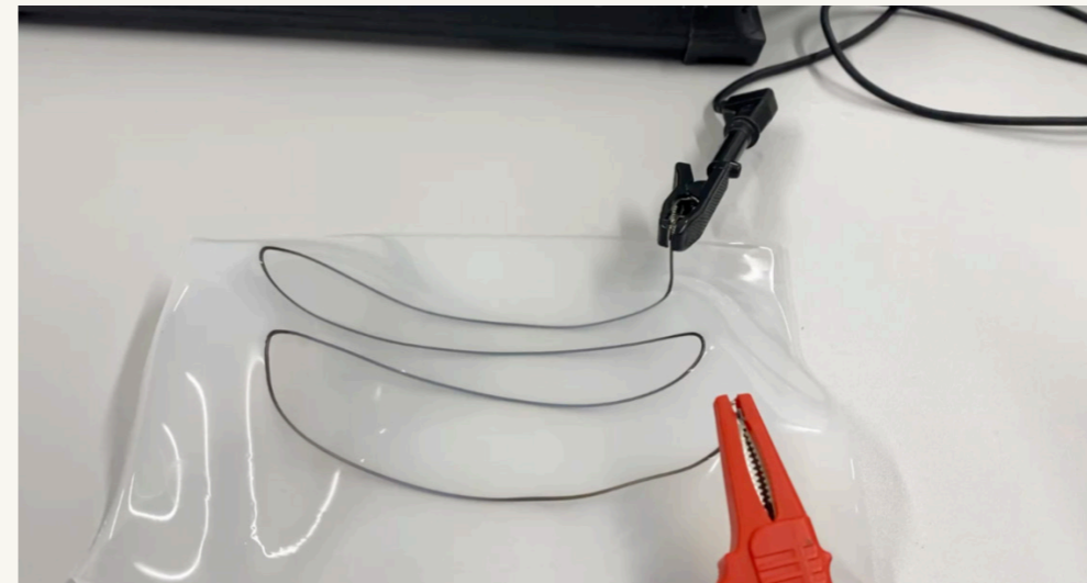
Figure 32: SMA wire embedded in silicon layer
