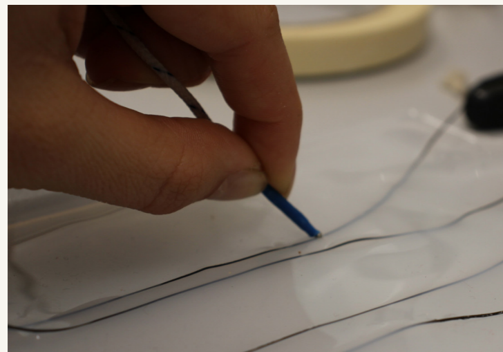
Figure 39: Thermocouple pressed on silicon
