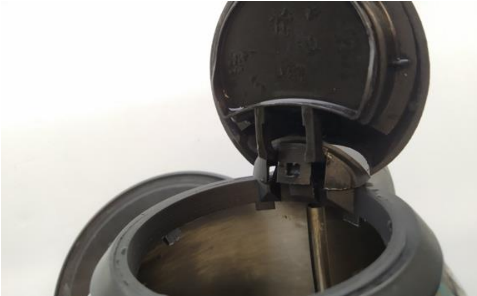
Figure 34 - Testing the fit and function of the top ring and switch inside the kettle.
