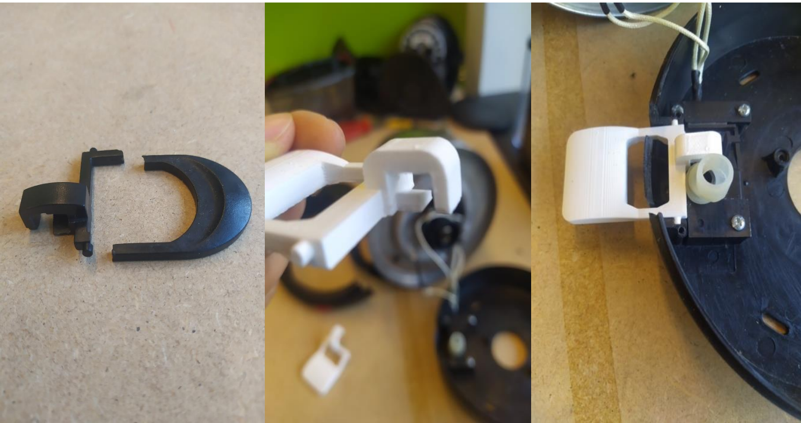
Figure 17 - Original IM part and installed FDM printed part. Case study: kettle switch.
