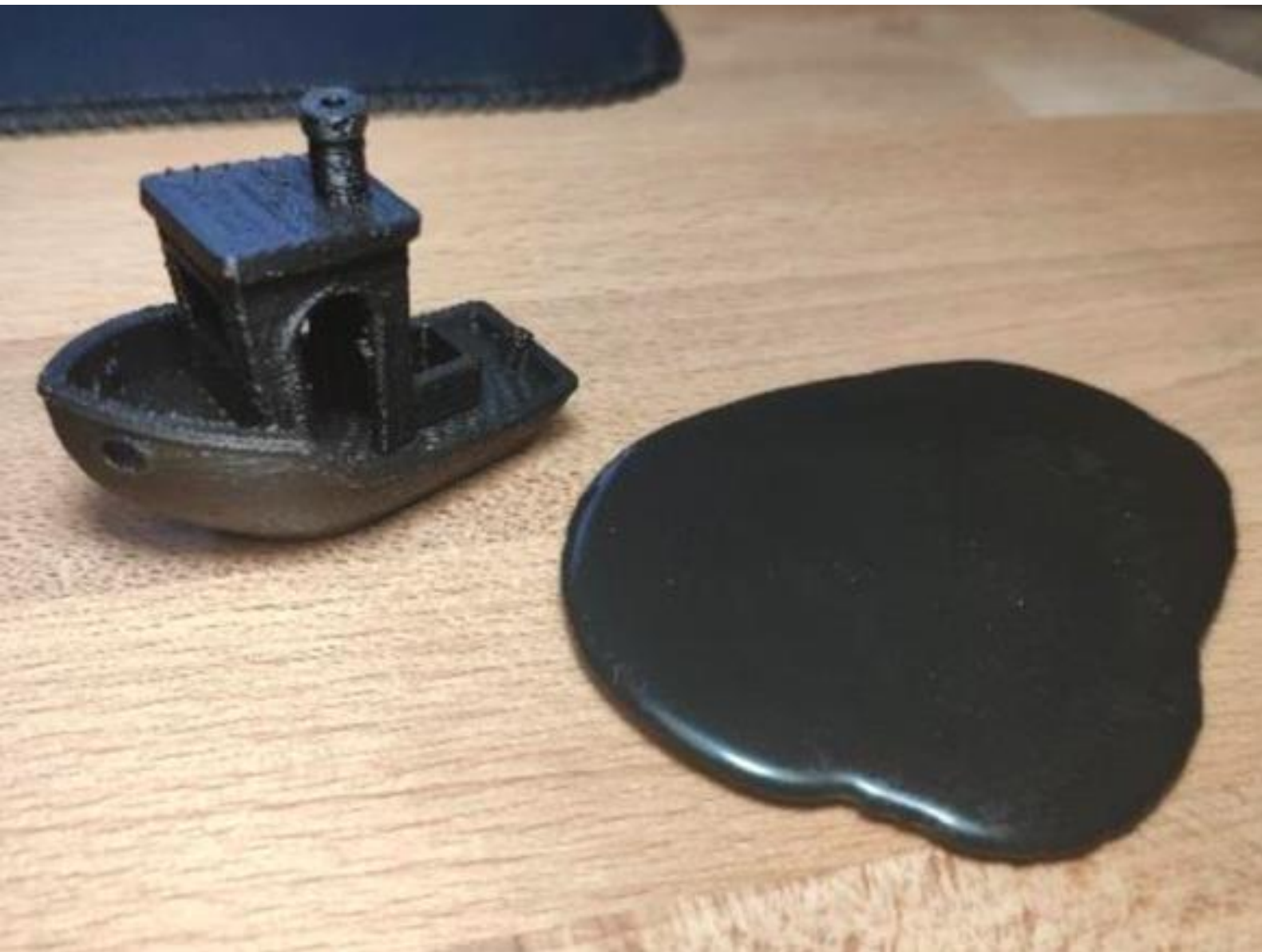
Figure 33 - Melted part after heat test. Used with approval of N. Van Silfhout, 2020.
