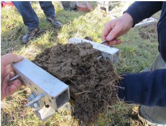
Figure 12 - Small pull frame which anchors the sod
