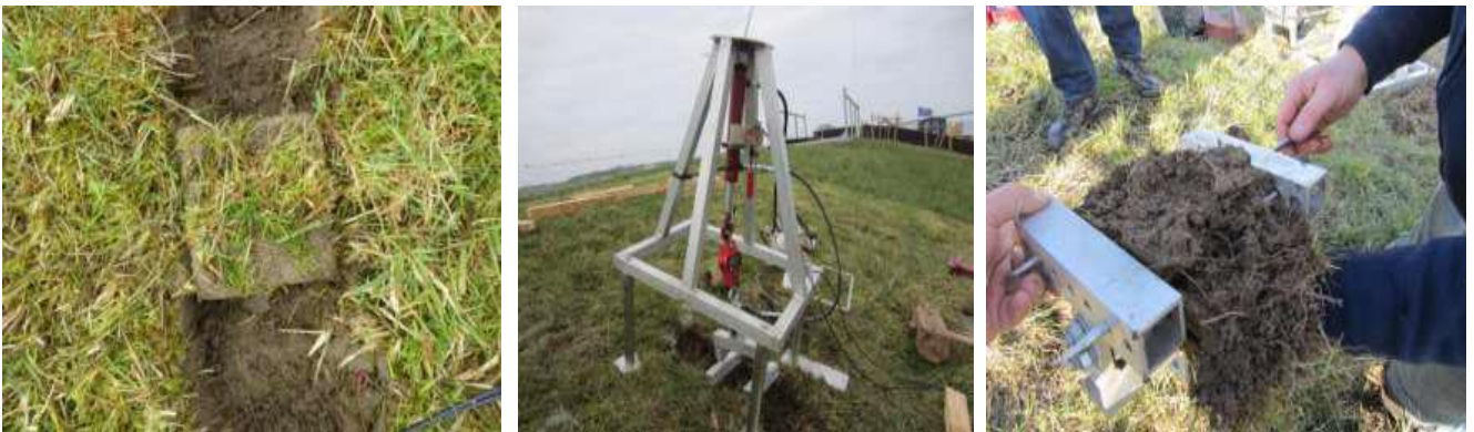
Figure 1a,b,c - Different stages during the sod pulling tests: Top view condition 4 test (a); Test set-up (b); Pulled out sod (c)
