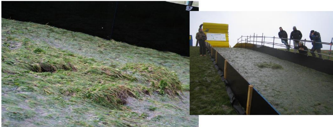
Figure 27 - Bulging of the grass sod during wave overtopping simulations (Infram 2008)
