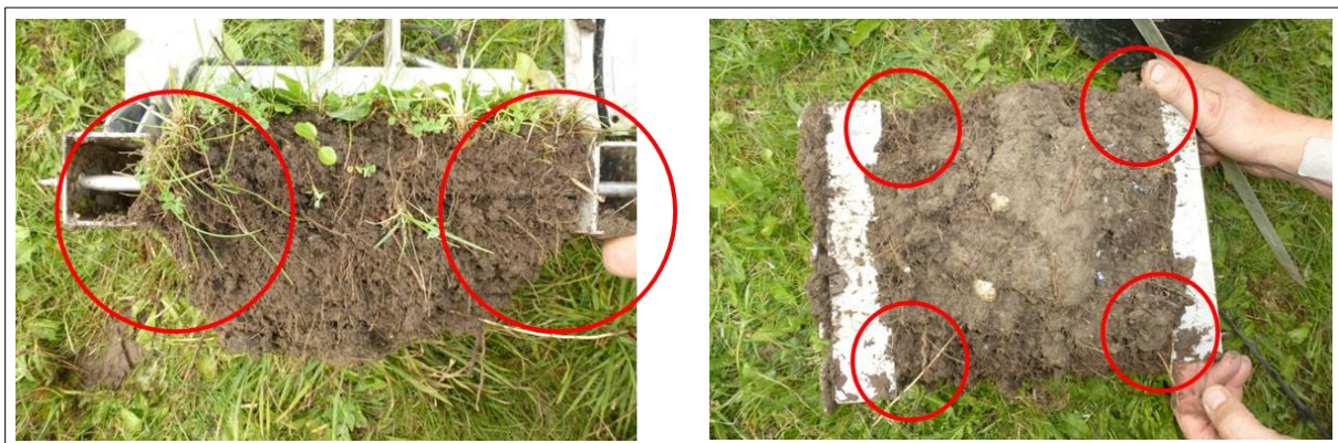
Figure 20 - Photos of the side and bottom view of missing corners due to the cutting
