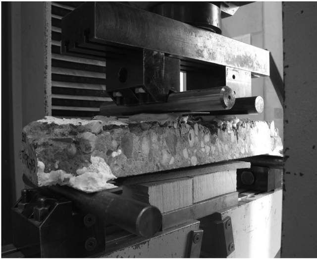
Figure 2. Test set-up used for four-point loading flexural tests.
