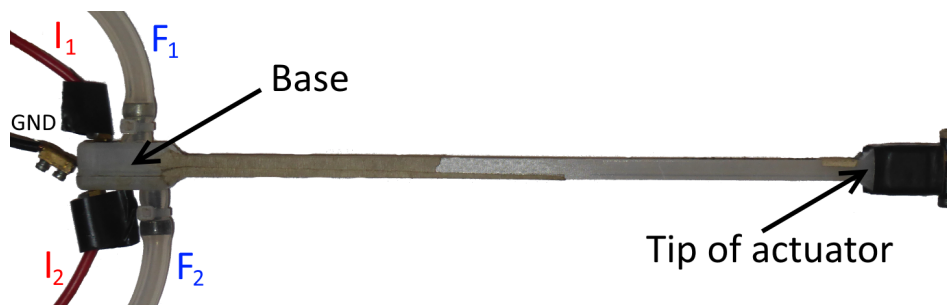
Figure A-1: Picture of the actuator with the connections indicated. The base indicates where the actuator is clamped into the setup and the tip of the actuator is where the deflection is measured.
