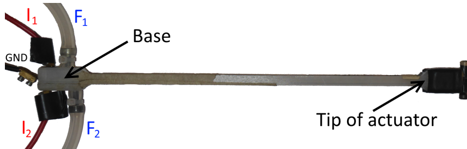
Figure 4-1: Picture of the actuator with the connections indicated. The base indicates where the actuator is clamped into the setup and the tip of the actuator is where the deflection is measured.
