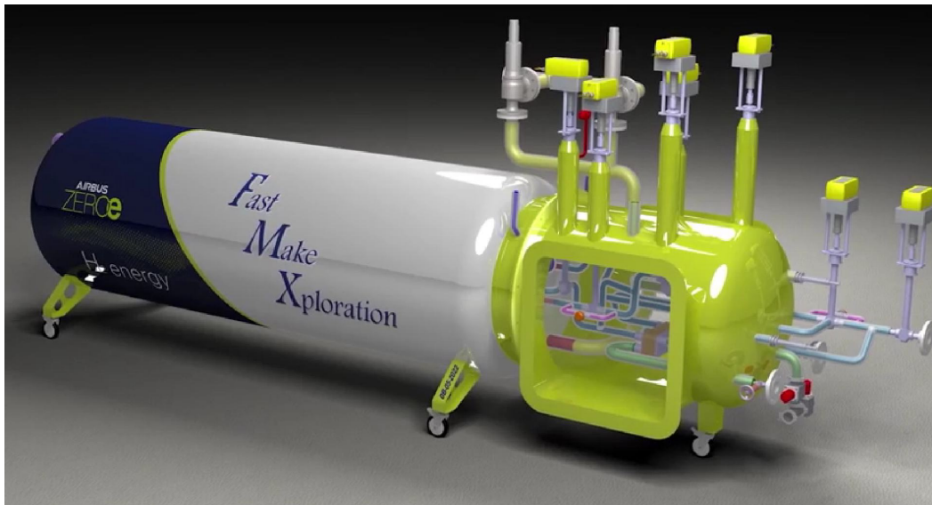
Figure 27: 3D drawing of the Fast Make tank prototype which could serve as a boundary object. (Airbus, n.d.)
