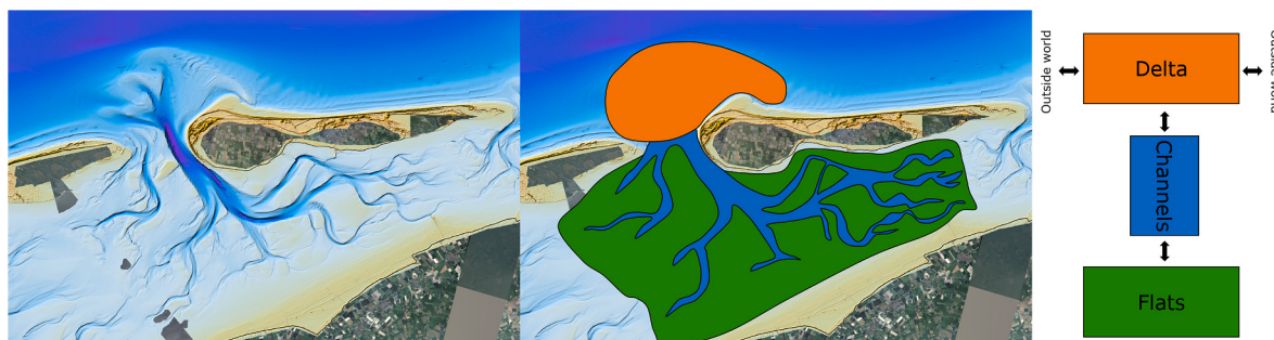
Fig. 2. Schematization of a tidal inlet system into a 3-element ASMITA model.
