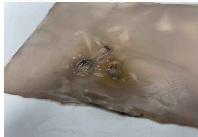
Figure 54 - Imprint of the copper wires in the cellulose sample
