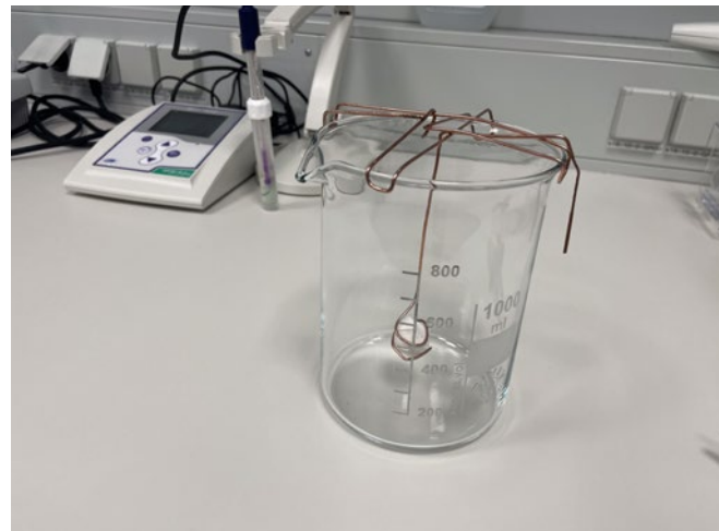
Figure 34 - Test setup with copper wire
