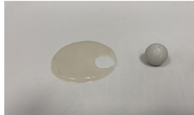
Figure 22- P1 test 1 resulting shape of DLP resin sphere
