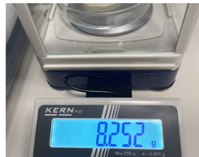
Figure 63 - Wet weight of the sample containing Tween80
