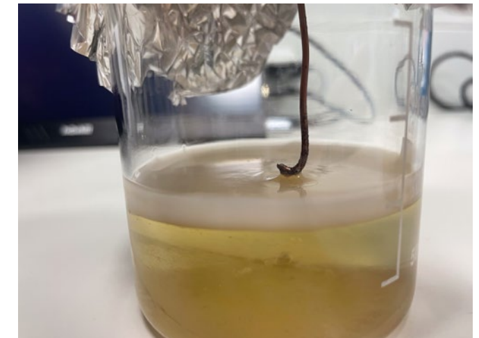
Figure 37- Copper wire touching the cellulose layer after day 4
