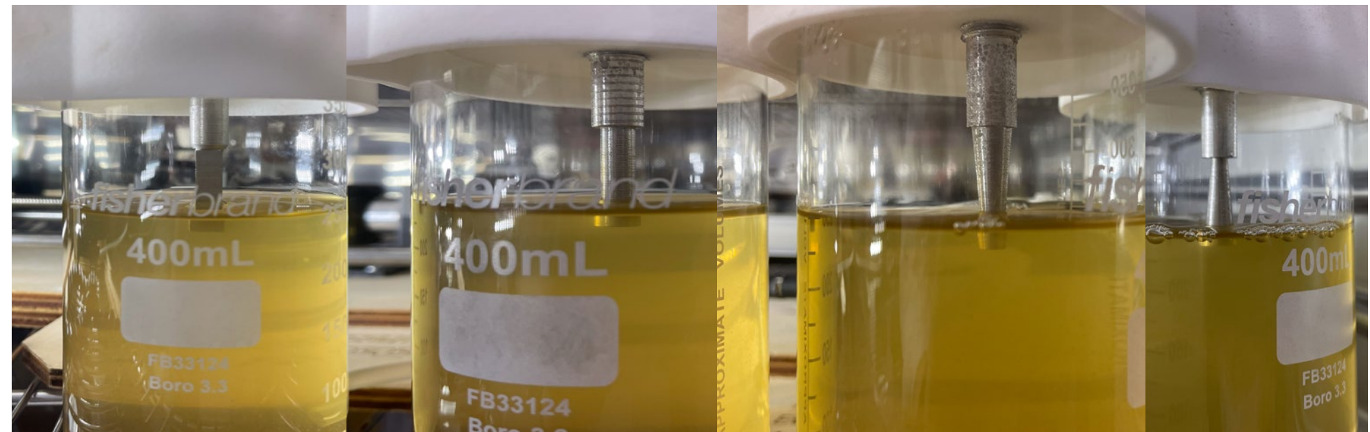
Figure 105 - Side view of the four geometries penetrating the air-liquid interface 5mm deep
