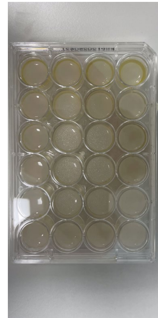
Figure 57 - 24-well plate containing CSL and oil
