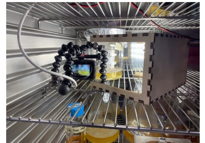
Figure 27 - GoPro setup monitoring the growth after day 4
