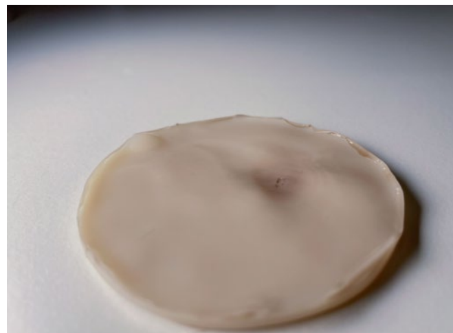
Figure 42 - Close-up of the cellulose sample showing the surface disturbances
