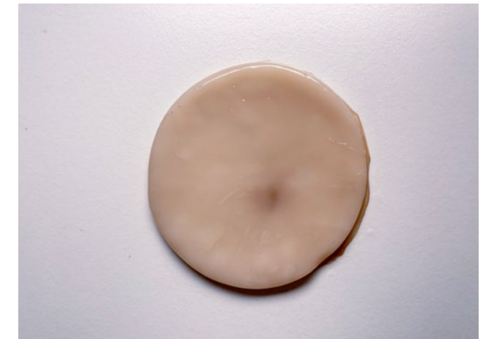
Figure 41 - Resulting cellulose sample after contact with copper wire (back)
