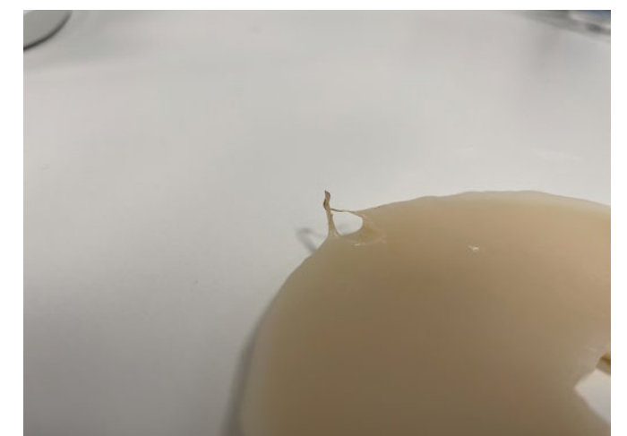
Figure 31 - Indent of the stamp in the extracted cellulose layer
