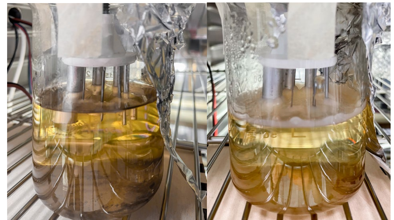
Figure 95 - The setup has reached State 2 at 48 hours, where loose clumps of cellulose are forming and capillary action is highly noticeable.
