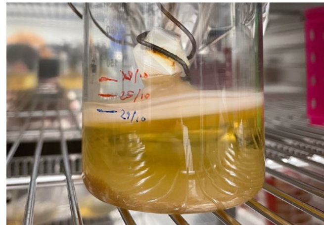
Figure 43 - Cellulose sticking to the geometry during the test
