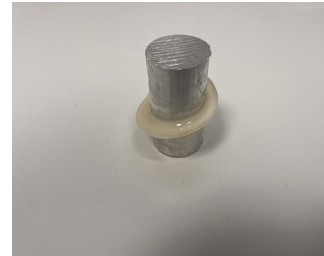
Figure 65 - Cellulose ring formed around the cylinder
