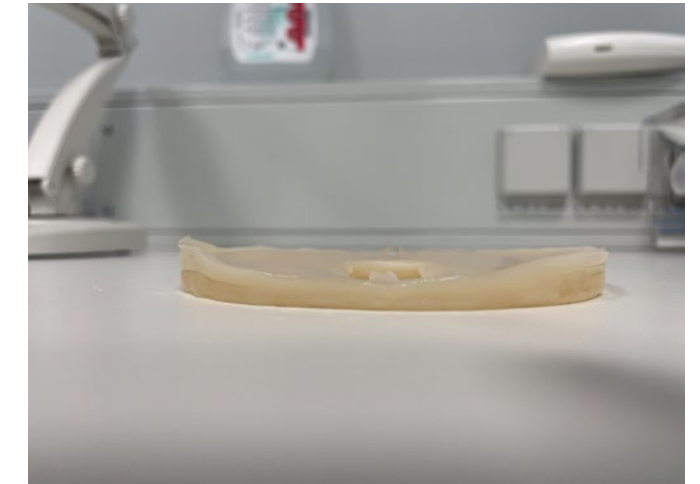
Figure 33 - Sideview of the cellulose layer showing the effect of the drooping
