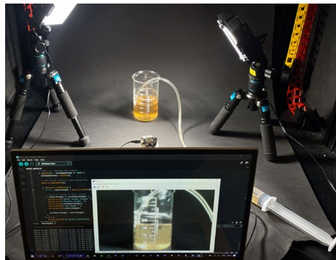
Figure 81 - Test setup for the evaluation of the image recognition camera
