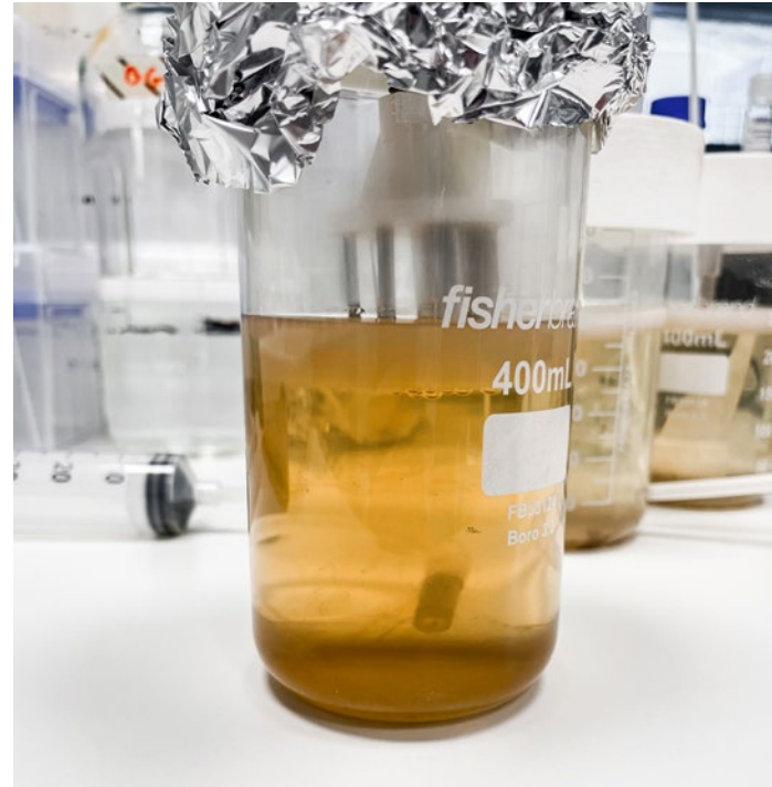
Figure 98 - Cellulose formation after 7 days of growth inside the vessel.
