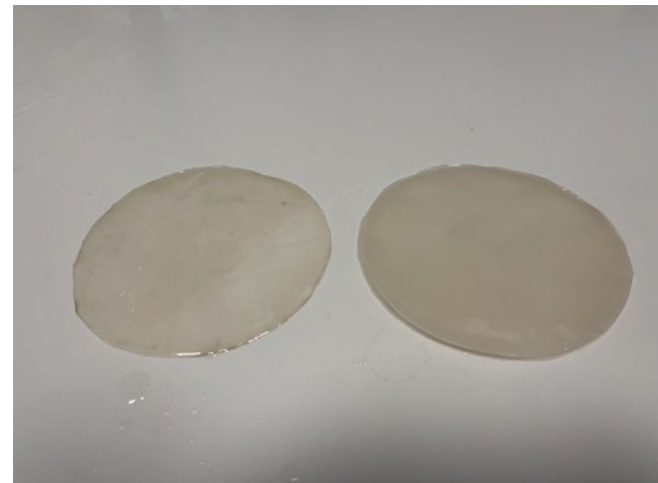
Figure 39 - Two separate layers of cellulose after addition of medium during growth
