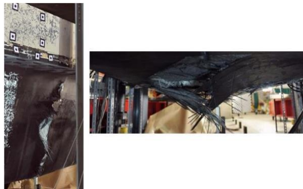
Figure 55 Shear buckling failure of beam (MARA, 2015)
