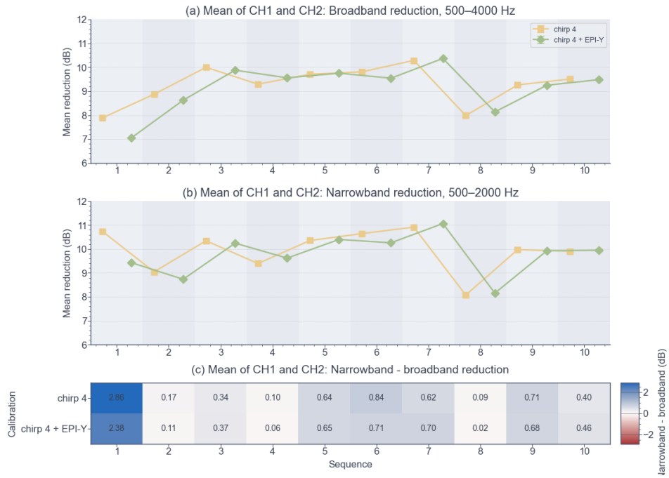
Figure 3.12: FFE mean reduction comparison for (a) broadband, (b) narrowband, and (c) narrowband - broadband chirp 4 vs. chirp 4 + EPI-Y calibration gradient.
