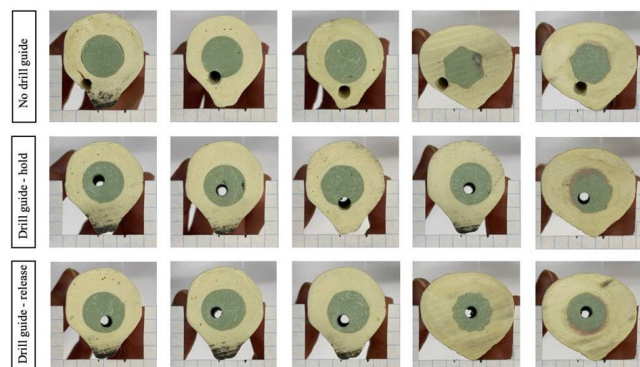
FIGURE 11. Drill hole locations at the cement plug exit point separated for the three different conditions.
