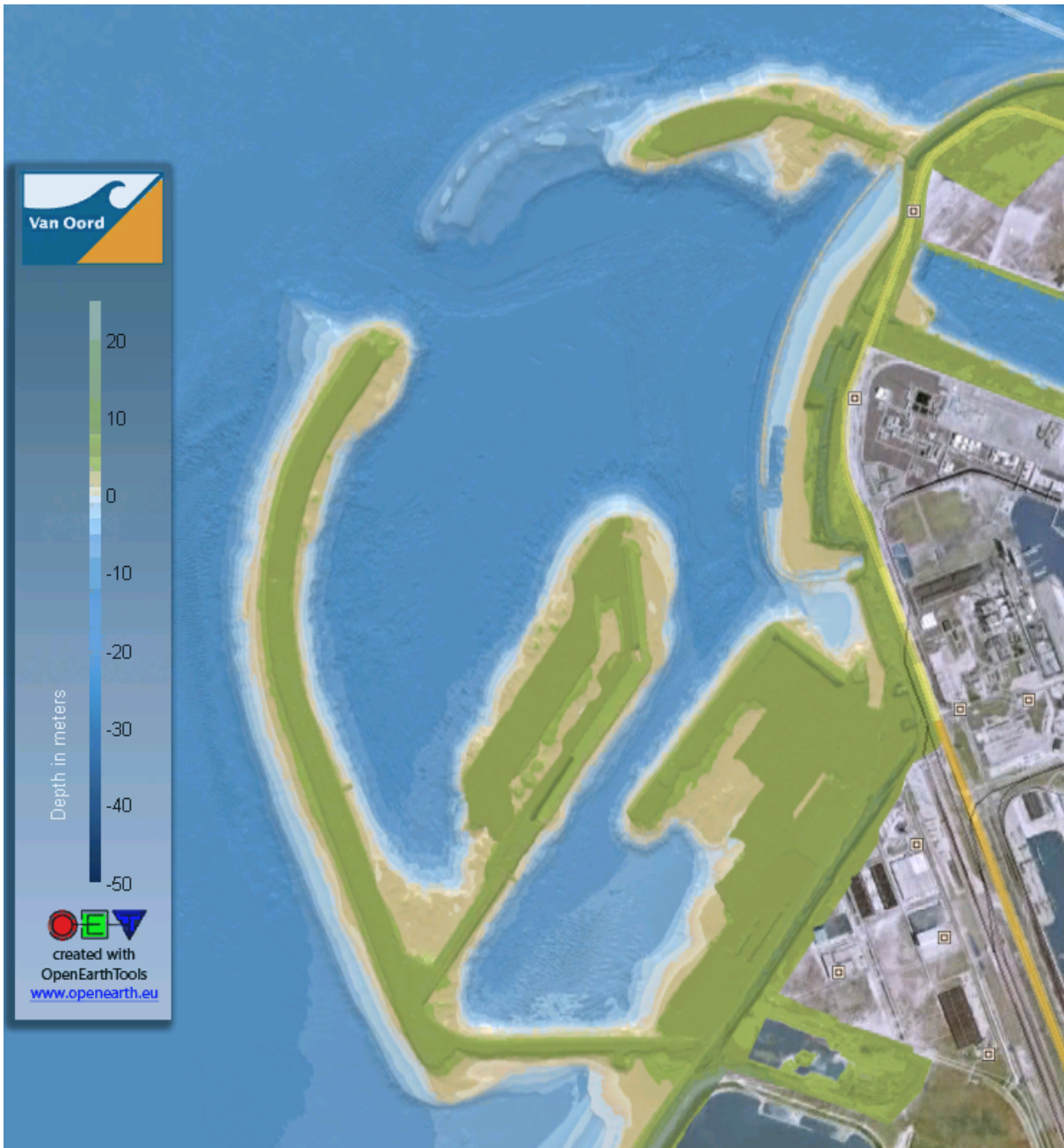
Figure H.15: Overview of the Maasvlakte II project. Survey data of May 31 th , 2010.
