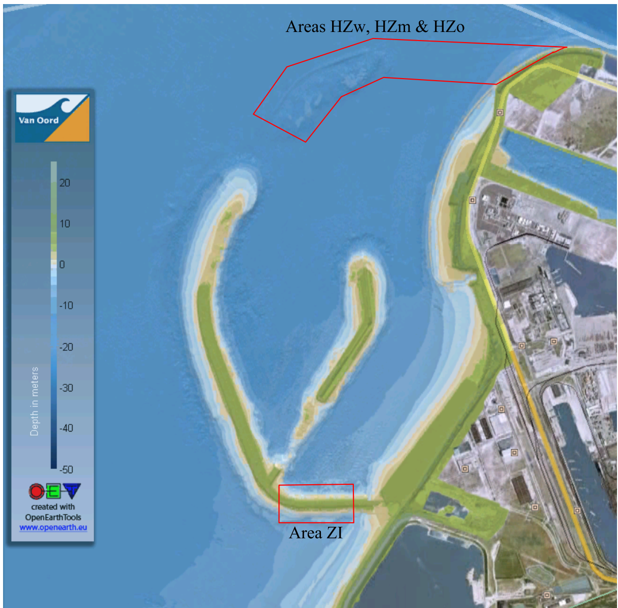
Figure H.8: Overview of the Maasvlakte II project. Survey data of November 1 st , 2009.
