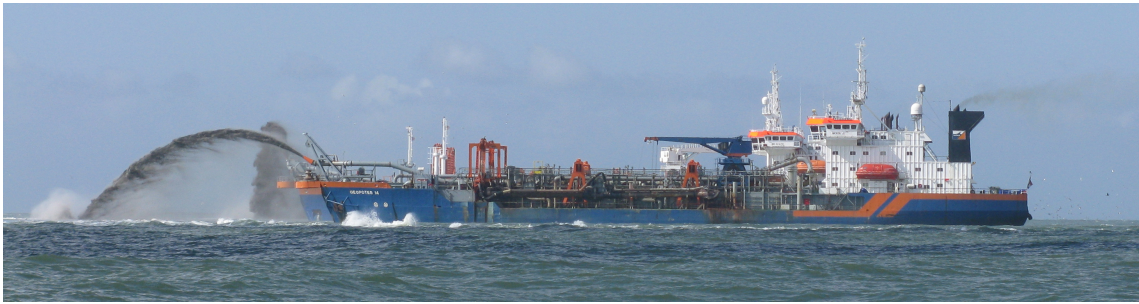
Figure 4.2: TSHD discharge method: rainbowing.
