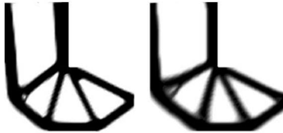
**Figure 2-8:** Optimized geometries for a classic L-bracket problem - Levelset based interface on the left, density based on the right with unphysical intermediate densities [James and Martins, 2012]
