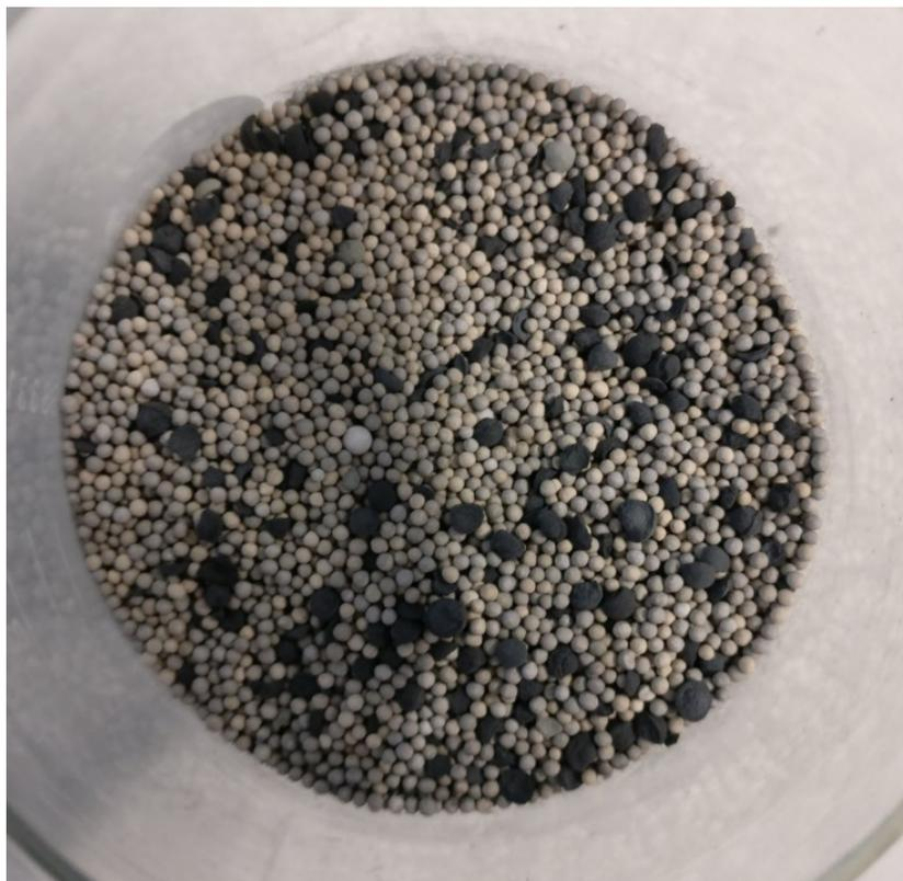
Figure 3.9: Combination of zeolite 4A/2,5mm Ni
