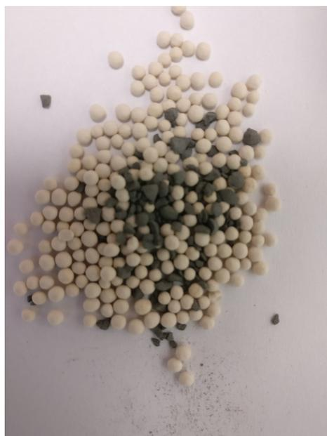
Figure 3.10: Combination of zeolite 4A/1mm Ni
