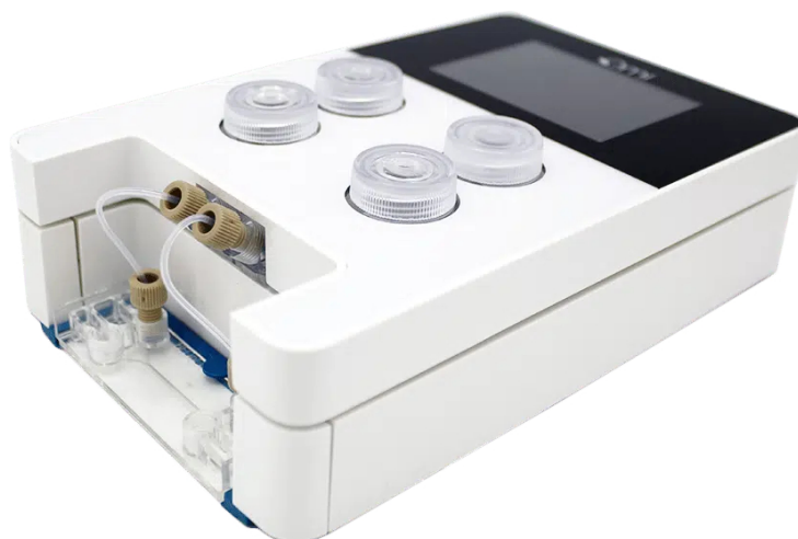
Figure 2.15: Omi microfluidic chip perfusion platform. Image courtesy: fluigent.com
