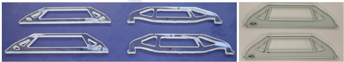
Fig. 16 Images of fabricated waterjet cut float glass beam specimen. The volume-based is on left, the stress-based is in middle, and in a separate photo the stiffness-based is on right
