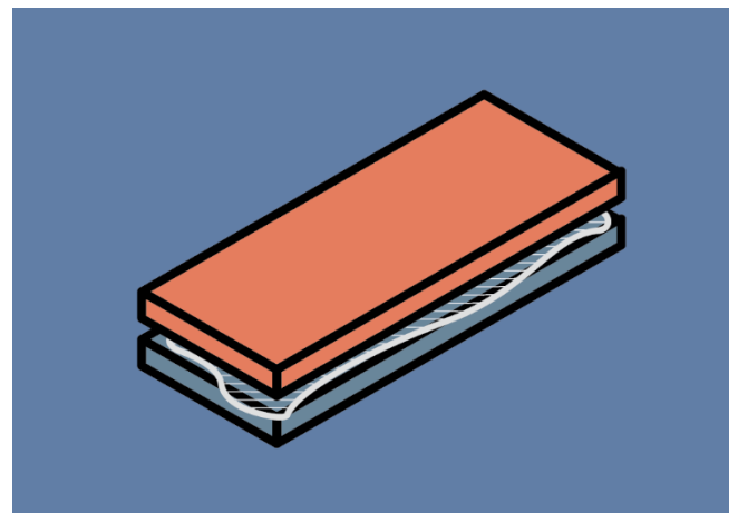
Figure 77: An adhesive joins two symmetric structures together
