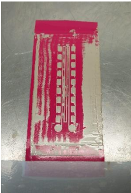
Figure 45: A substrate with stencil after the print. Excess silver paste collects in the inconsistencies of the substrate
