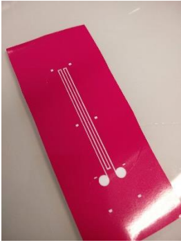
Figure 44: A substrate covered with a vinyl stencil containing a positive of the trace
