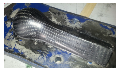
(b) Carbon fiber X-Core gearstick marking the first product produced with X-Core
