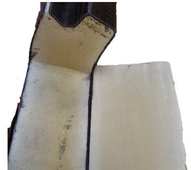
Figure 8.35: Comparison of discoloration seen in a prototype doorbeam (left) with 146^\circ\text{C} predicted core-temperature to a tile mould sample (right) with 154^\circ\text{C} core-temperature
