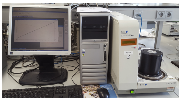
(a) Seiko Instruments Exstar 6000 DSC with computer used for data collection
