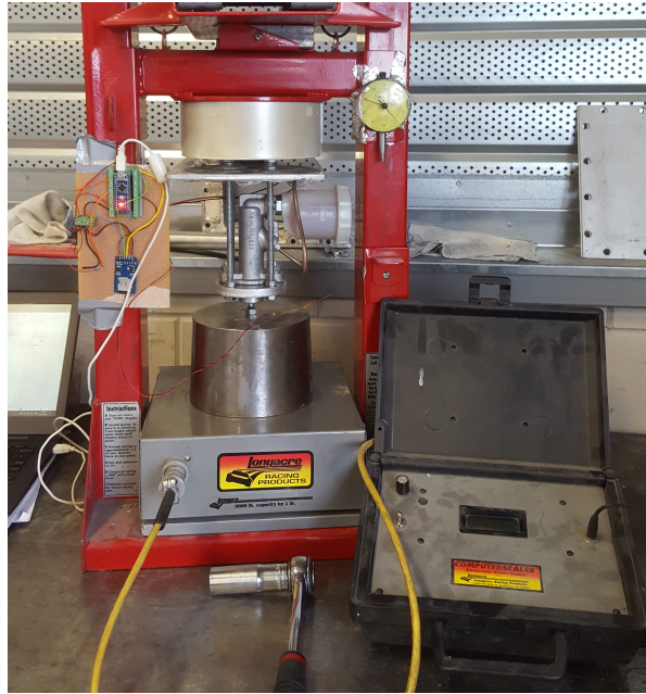
Figure D.2: Master cylinder placed inside the Donkervoort pressure jack with 1lbs accurate load cell underneath.
