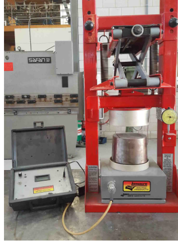
Figure 4.5: Pressure jack with load cell underneath and readout display combined with dial gauge micrometer [22]
