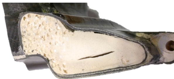
Figure 3.5: Cracking of X-Core observed in region with pure DE/DU resin blend linked to exothermic temperature peaks
