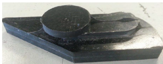
(a) One-shot manufactured complex shaped sandwich structure with carbon facesheets and X-Core core material
