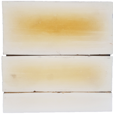
Figure 7.3: Cross-sections of X-Core samples of 80 (top), 55 (middle) and 30mm (bottom) height. Discolouration visible relative to maximal temperatures present in the central region of the sample which reached 167, 154 and 130°C respectively.
