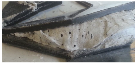
Figure 3.2: Result of the re-heating of a cured pure DU/DE Expancel blend sample with carbon fiber facesheet
