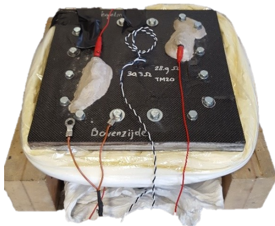
(a) Tile mould with breather cloth wrapped around the aluminium walls as insulation band (white)
