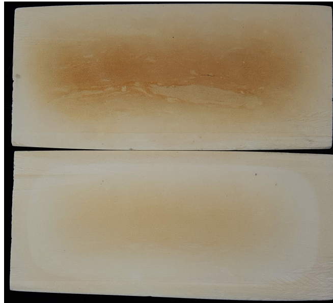
Figure 7.15: A series sample cross section (top). Discoloration visible with micro-cracks appearing in the high temperature region. Region of discolouration closely corresponding with temperature distribution shown in figure 7.6. B series sample cross section (bottom). Less discolouration visible in centre region compared to A sample linked to lower maximal core temperatures. Distinct darker region around the outer edges indicative of possible high resin concentrations
