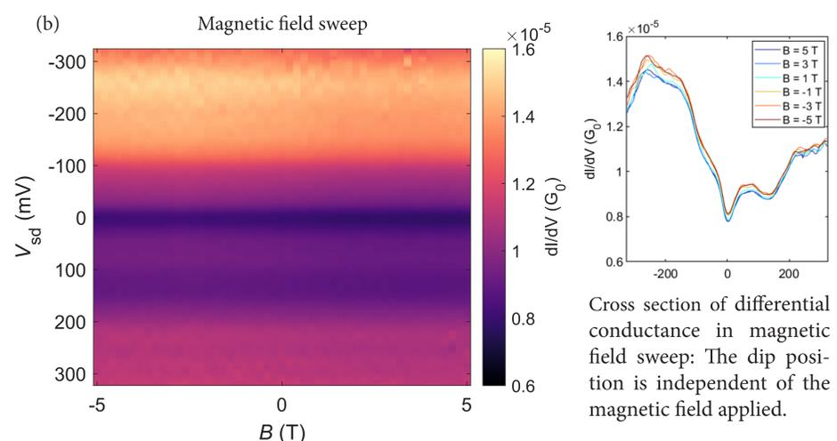
Cross section of differential conductance in magnetic field sweep: The dip position is independent of the magnetic field applied.
