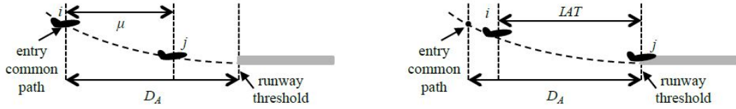
Figure 2.2: Time separation between a following aircraft i and leading aircraft j , at the entry at the common path of following aircraft i and at touch down of leading aircraft j [27]
