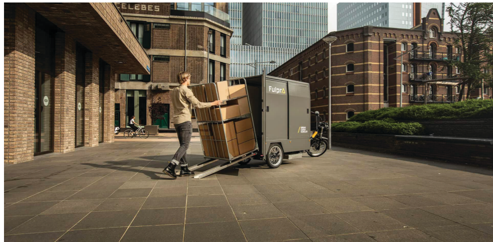
Fulpra bikes are made to carry specially designed racks. The bikes have a load capacity of 3000L / 350kg
