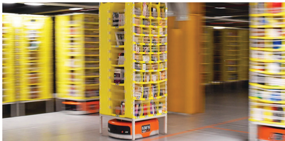
Amazon robotics are made to move around specially designed racks in the fulfilment centre
