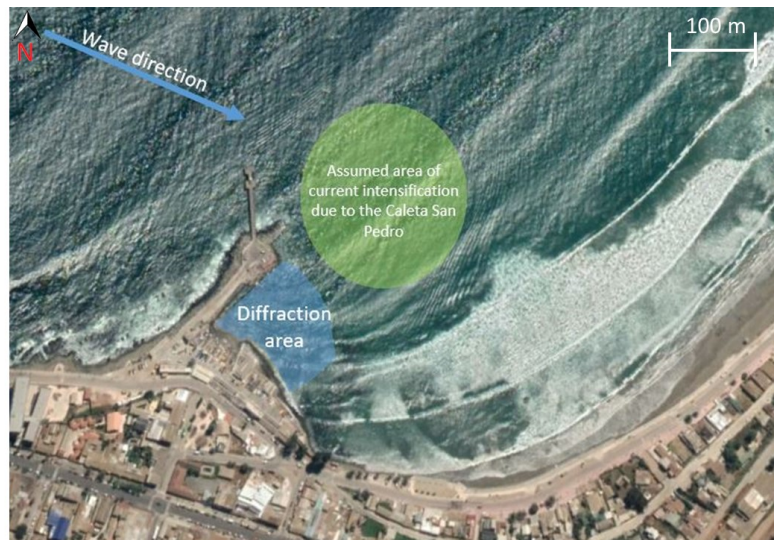
Figure 5.36: Influence of the Caleta San Pedro on the waves and currents (GHD, 2016c)
