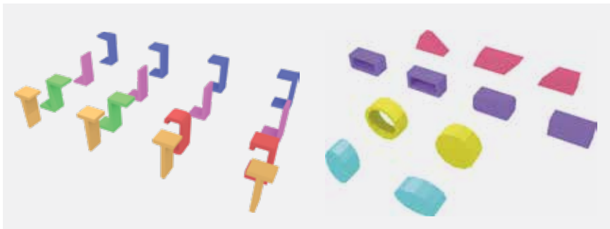
Figure 2: IFC has several predefined parametric profiles, such as those based on the characters U, L, Z, C and T (left) or based on trapezoids, rectangles, circles and ellipsoids (right).
