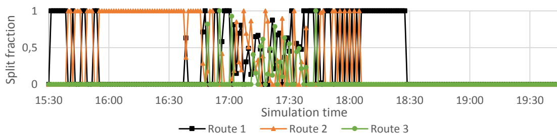
Figure 5.38: Split fractions induced by the controller at the first A2 decision node in the high demand scenario. Route 1 via links 2-3-4-6-7; Route 2 via links 2-3-8-9-10; Route 3 via links 11-12-9-10
