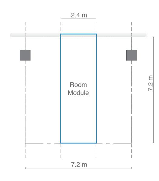
Floor to ceiling height = 3.2m Orientation = West Room volume = 55.30 $m^3$ Room floor area = 17.28 $m^2$ Indoor set point temperature = 26.7  $^{\circ}C$ Indoor set point RH% = 60 %
