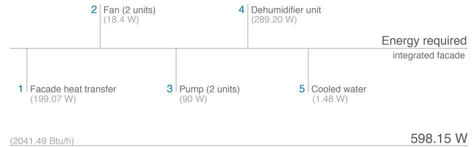
$H_{facade} + H_{fan} + H_{pump} + H_{dehumidifier} + H_{cooled water}$  required energy for integrated facade
