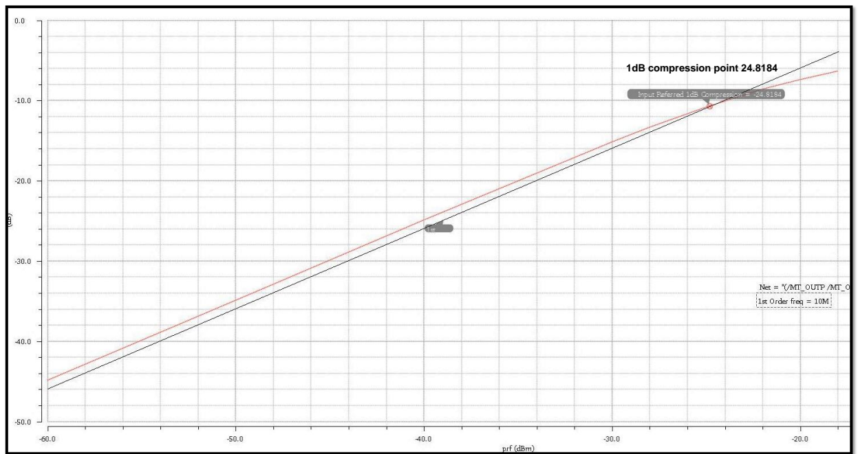
Figure 5-3: Simulation results of the mixer - input referred 1 dB compression point.
