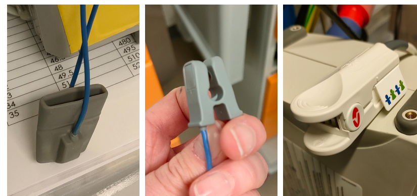
Figure 2.8: the reusable Philips glove sensor (left) and ear-clip (middle) and Masimo clip sensor (right)
