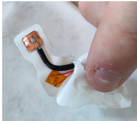
Figure 2.2: components of a disposable pulse oximeter
