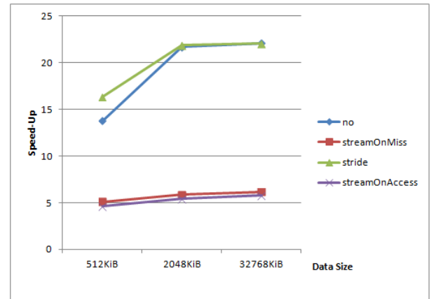
Figure 4.24: Speed-up of the Ideal Prefetcher when the sentence's first letter capitalisation algorithm is executed on the OOO core over the reference prefetchers as the input size increases
