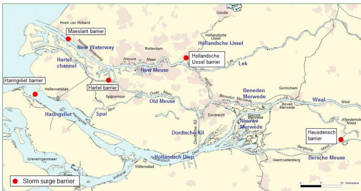
Figure 6: Current water-system with water barriers. (RWS (adapted))
