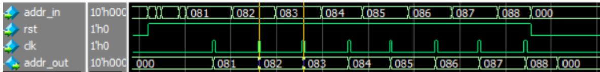
Figure 5.4: Waveform of the transmitter's output
