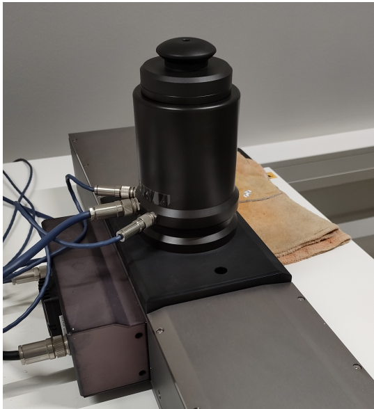
(a) Picture of the exterior of the Hall-effect measurement setup
