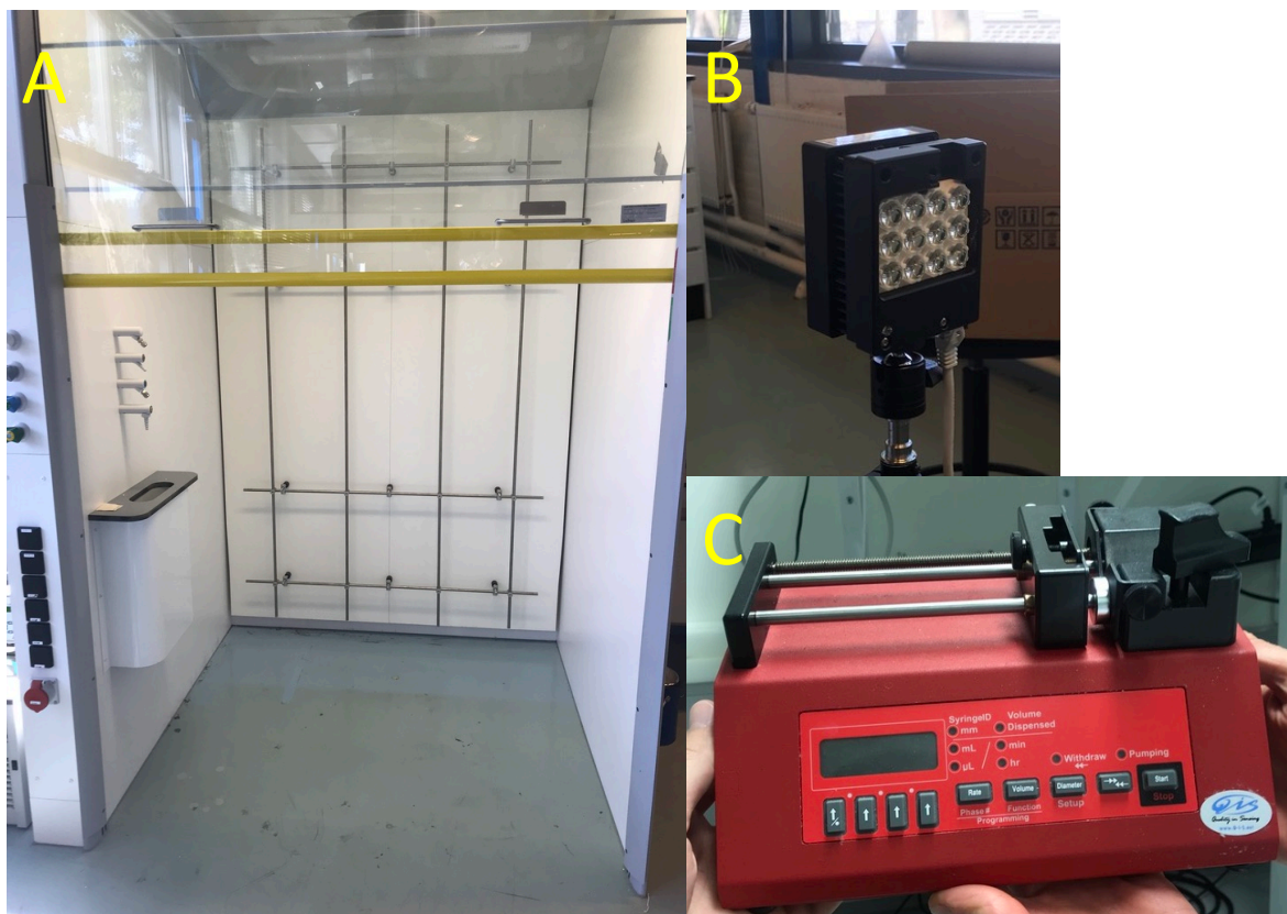
Figure C.1: A- Fumehood used for the tests at the Chemical lab of the DASML. B- Lighting system for high speed camera. C-Syringe pump used for drop-test experiments
