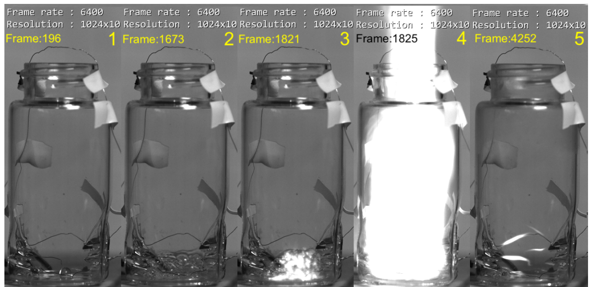
Figure 5.13: Image sequence recorded with High Speed Camera at 6400 fps of ignition sequence of 95% HTP falling on gelled EtOH with 1.8% wt. gelling agent for gellation. The temperature profile as well as the numbering can be seen in Figure 5.14. FTK2 was melted in the previous experiment and can be seen cut in two. 1- 95% HTP falling onto the bottom of the VES, gelled EtOH is already there on the left on the HTP droplet ( frame:96 ). 2- Caging phenomena typical of gels starts to take place after HTP starts to interact with it ( frame:1673 ). 3- Ignition takes place, IDT calculated until here and equal to 253.9 ms ( frame:1821 ). 4- Full spread of ignition across the entire vessel, signs of throat-like behavior can be seen ( frame:1825 ). 5- Signs of continued combustion of the ignited gelled EtOH, as the FTK still glow due to the heat released of the remaining gel ( frame:4252 ).
