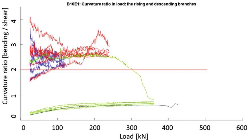
**Fig. 6.** Curvature ratio plotted against the applied load in test B10E1 (load stages are indicated in different colours: blue – 1st load level cycle, red – 2nd load level cycle, green – 3rd load level cycle).
