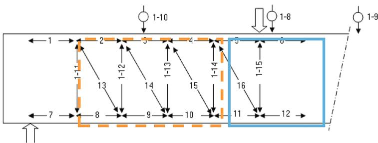
**Fig. 1.** The test setup of the specimen B10E1, LVDT sensors numbered. Blocks indicate the specimens shear zone (orange-dashed) and bending zone (blue).
