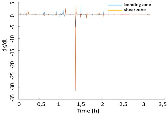
Fig. 5. Tangential stiffness development in time in test B10E1.
