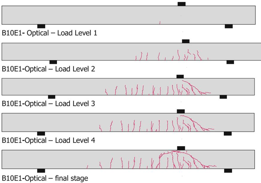
Fig. 7. Crack development in test B10E1 (Uijl den).
