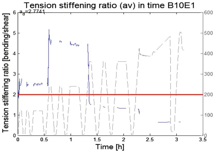
Fig. 8. Tension stiffening for the filtered load data in test B10E1.
