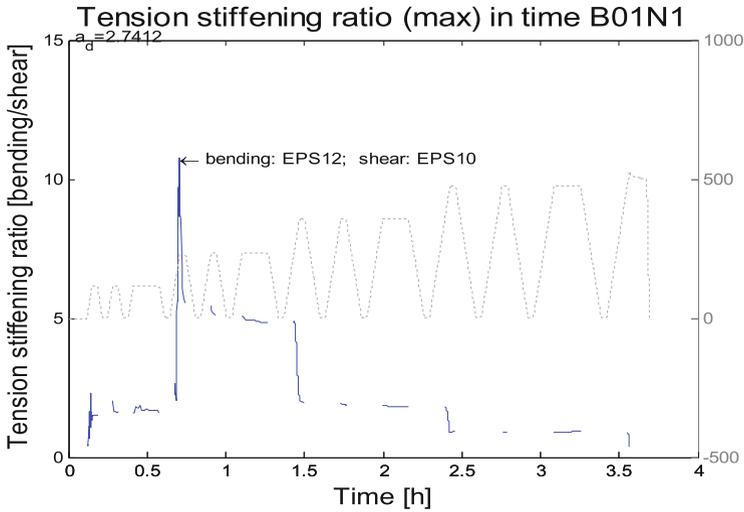
**Fig. 9.** Tension stiffening for the filtered load data of B01N1.
