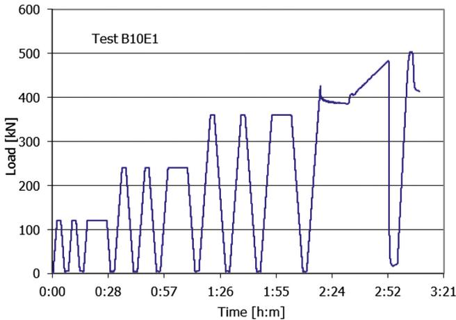
**Fig. 2.** Loading scheme of B10E1.
