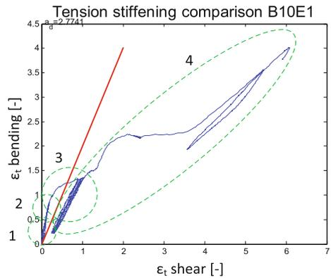
**Fig. 4.** The relation between curvature in the bending and shear zone, green circles correspond with the applied load step.
