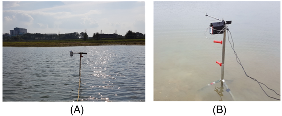
FIGURE 3 (A) Broadband (285–2,800 nm), and (B) spectrally resolved (278–1098 nm) albedo measurements at two different spots in the pond [Colour figure can be viewed at wileyonlinelibrary.com ]
