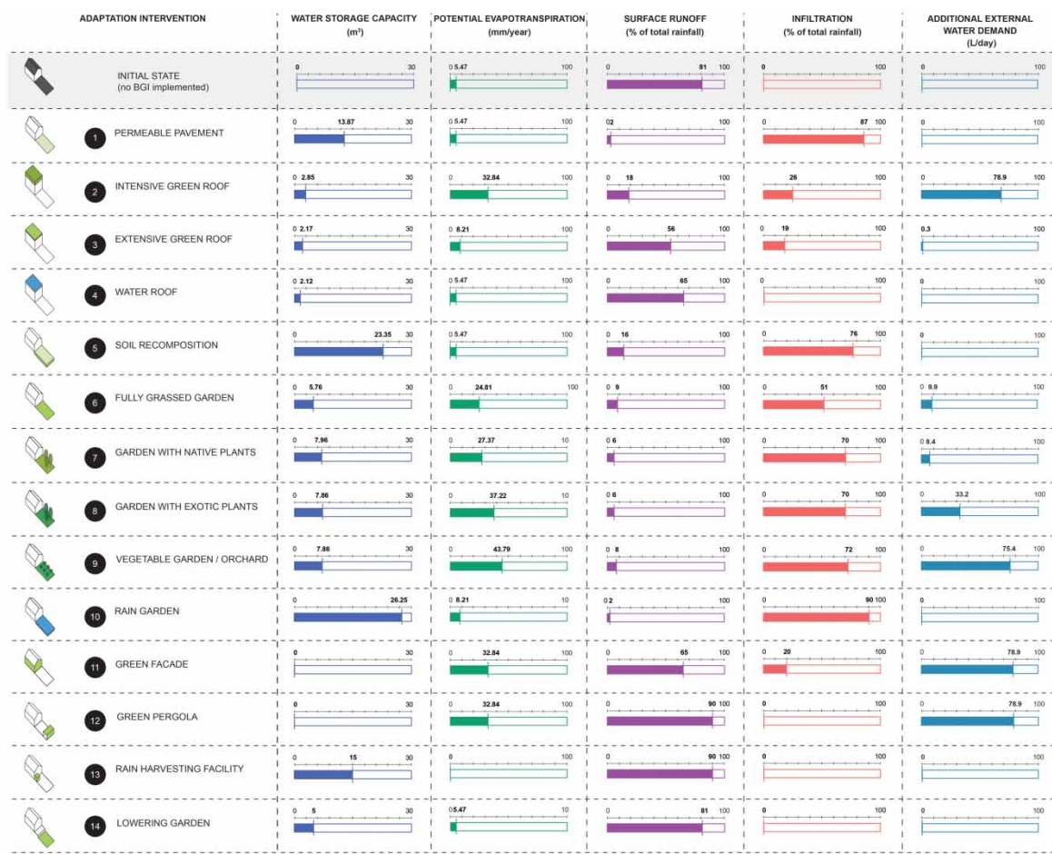
Figure 3 | (a) BGI impact metrics. The top row shows the baseline (original house setup). The remaining rows show 14 individual BGI types, each applied separately per application area (roof, garden, or facade). Columns present water balance indicators. (b) BGI impact metrics. The top row shows the baseline (original house setup). The remaining rows show 14 individual BGI types, each applied separately per application area (roof, garden, or facade). Columns present co-benefit indicators. (continued).
