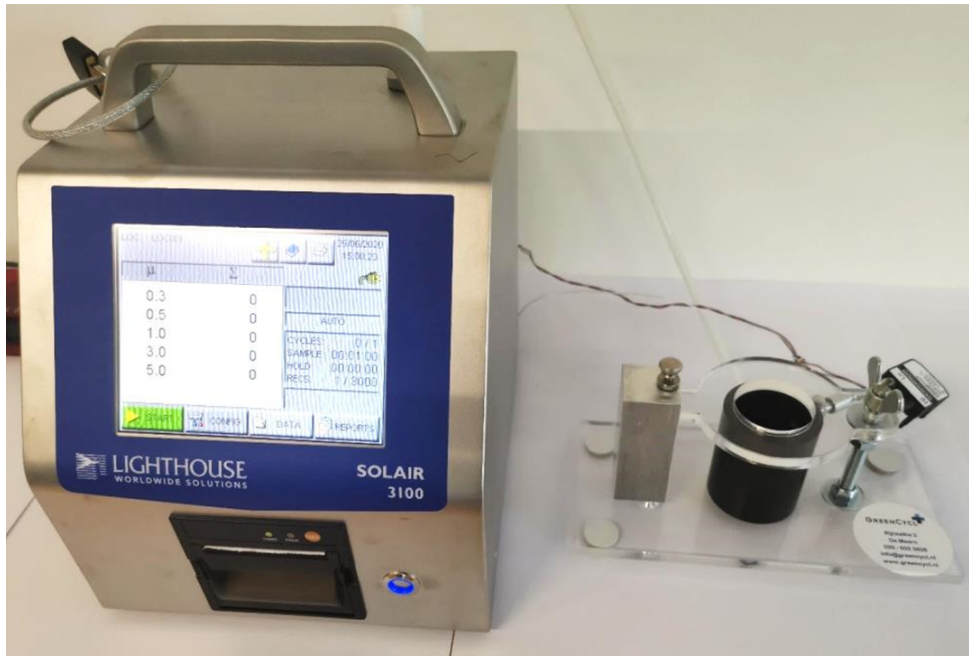
Figure 7.2: Lighthouse Solair 3100 particle counter connected to a particle chamber.
