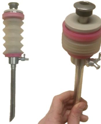
Figure 8.4: The redesigned trocar with the extendable bellows
